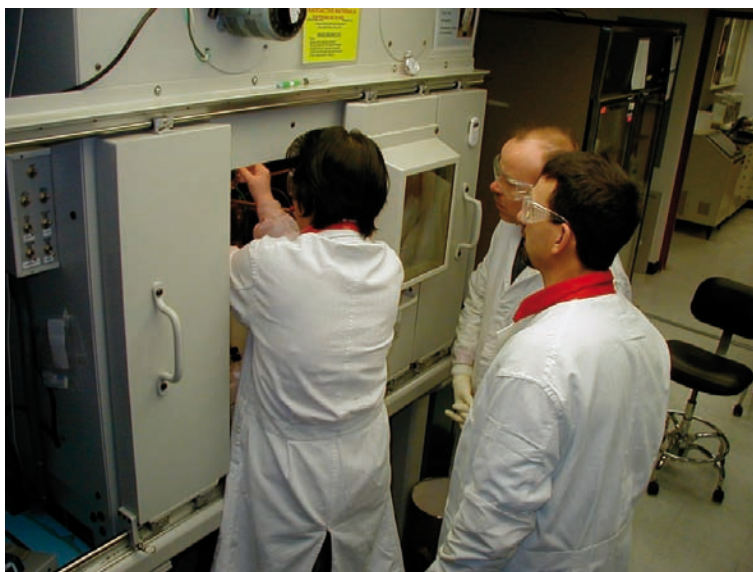
FIG. 4.1. Sliding leaded glass shield hot cell design.
