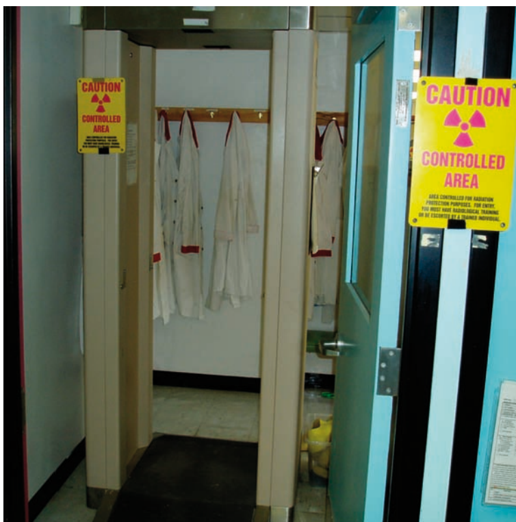
FIG. 9.4. Example of a whole body checking station inside a laboratory doorway. Note the postings on the outside of the laboratory.
