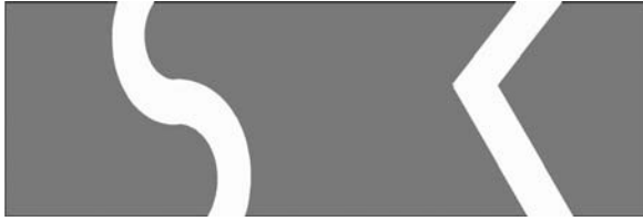
FIG. 3.4. Examples of shielding wall penetrations designed to minimize line of sight radiation.
