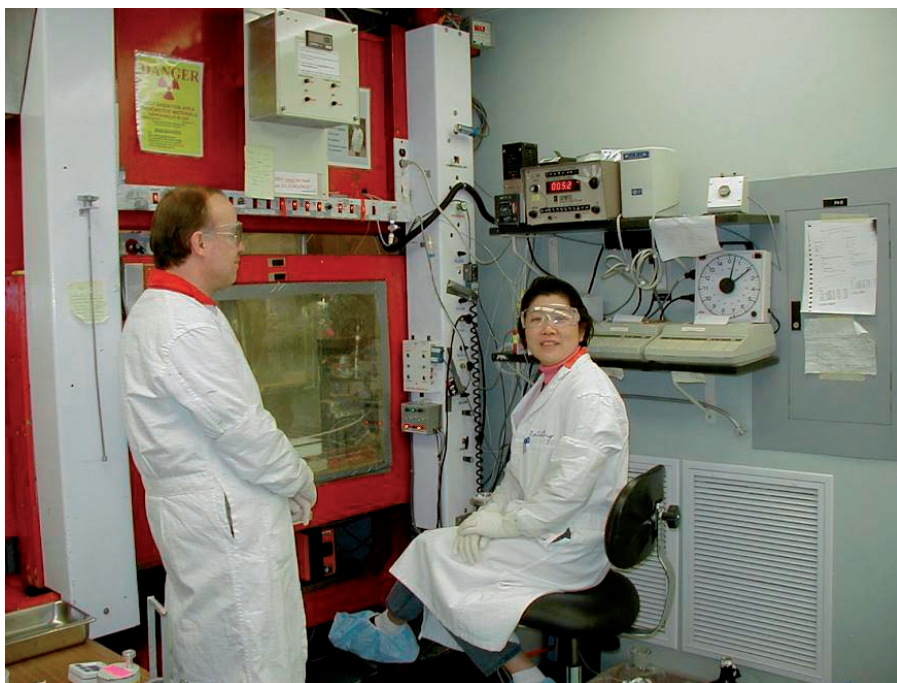
FIG. 1.11. Hot cell with leaded glass window that can be lowered for working inside when radioactivity is not present.
