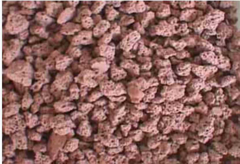
FIG.5. Granulated heavy spar bonded in Geopolymer ®
