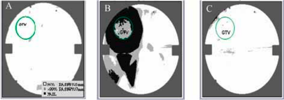
FIG. 4. BAM plots for Pinnacle SC (A), Eclipse PB (B) and Eclipse AAA (C) heterogeneity corrected dose calculations compared to measured dose distributions in a thorax phantom using a \pm 5\%/3 mm criteria.
