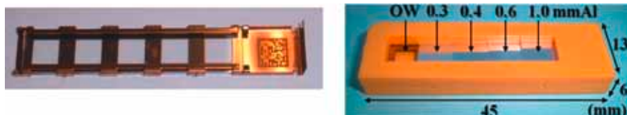
FIG. 3. Photograph of a glass dosimeter for mammography radiation: glass plate (left) and case (right).
