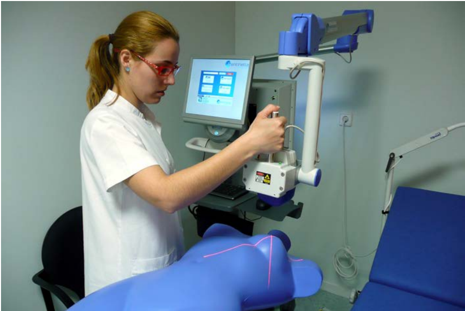
FIG. 5.10. Sentinella 102 (Oncovision, Valencia, Spain) is a portable gamma camera fitted with a pinhole collimator designed for intraoperative use. A laser pointer centres the target image on the screen.
