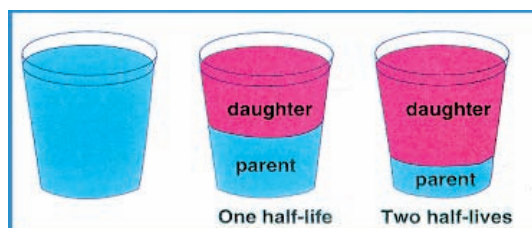
FIG. 3. Schematic illustration of the radioactive decay of a radionuclide into a nuclide of another element, or daughter.
