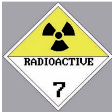
FIG. 15. Placard design. The number 7 is the UN hazard class number, which indicates the presence of radioactive material.
