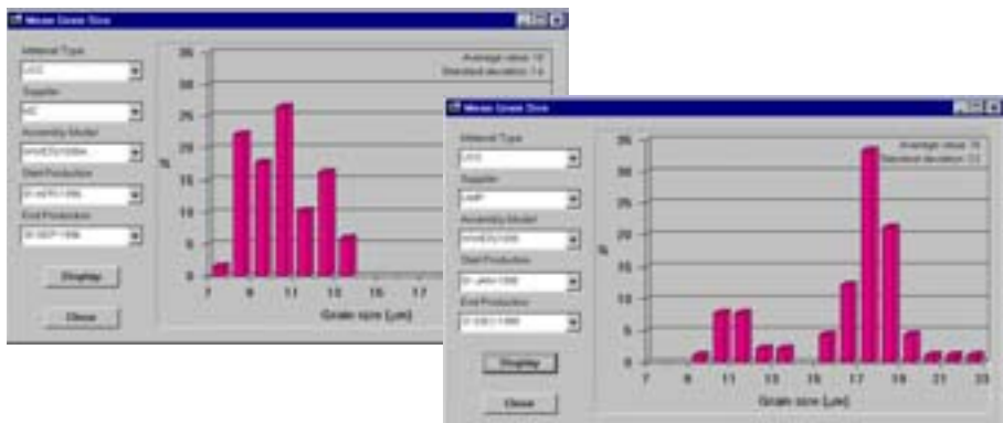
FIG. 1. Distributions of mean grain size for WWER-1000 fuel pellets of various origins.
