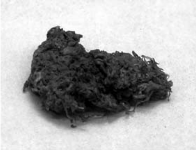
FIG. 3. Cellulose material, originating from a reinforced wiping cloth.
