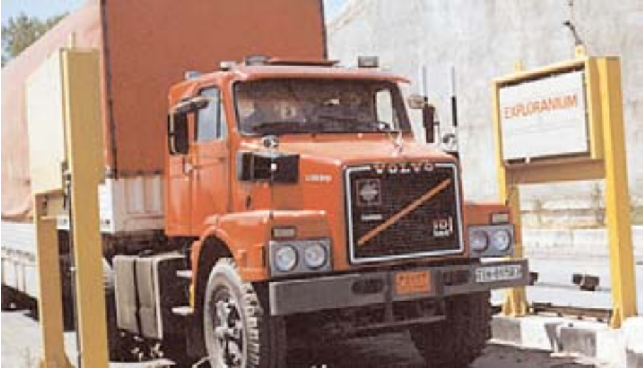
FIG 2. A gamma scanning gate monitor at a border crossing at Astara (Exploranium system).
