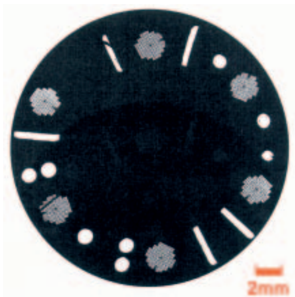
FIG. 1. The sample used in the IAEA–ITU experiment: pyrolytic carbon planchet with U_3O_8 particles at centre, vacuum deposited 6 ‘finder’ grid Cu thin film patterns, and orientation signs. The image is a photomontage of SEM-BSE images. The particles at the centre are hardly visible at this low magnification.
