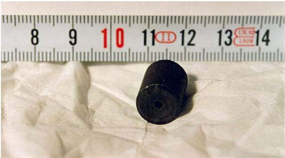
FIG. 1. A uranium oxide fuel pellet from a seizure of material in Munich in 1994 identified from its form, diameter and height, and the presence of a central hole, as a pellet intended for use as fuel in an RBMK reactor.
