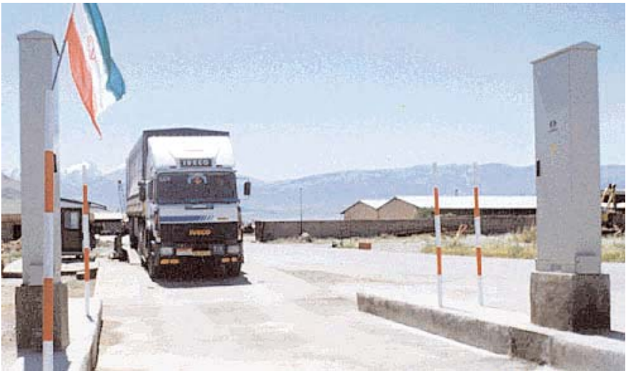
FIG. 3. A gamma scanning gate monitor at a border crossing at Jolfa (Rados system).
