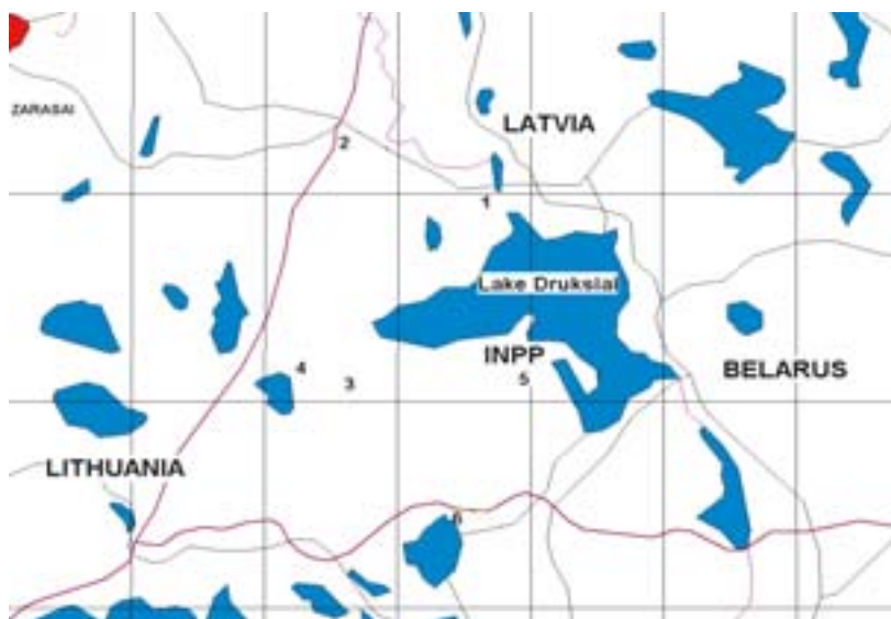
FIG. 2. Map of the Ignalina NPP site showing locations of air samplers. For details see Table I.
