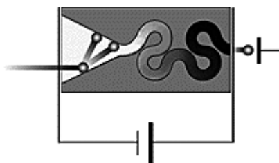
FIG. 1. Schematic of an ion striking a CDEM detector (source: Sjuts Optotechnik GmbH).
