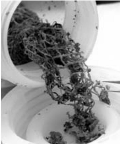
FIG. 2. Nylon netting, originating from a reinforced wiping cloth.
