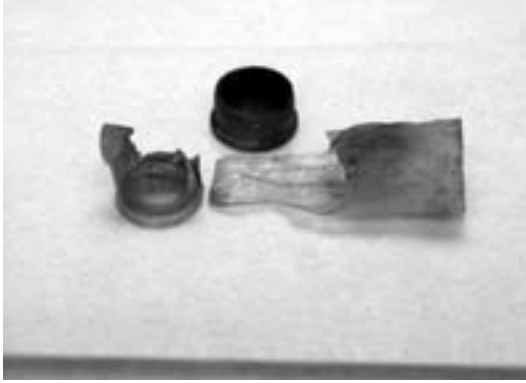
FIG. 1. Broken plastic vial, showing brownish radioactive residue.
