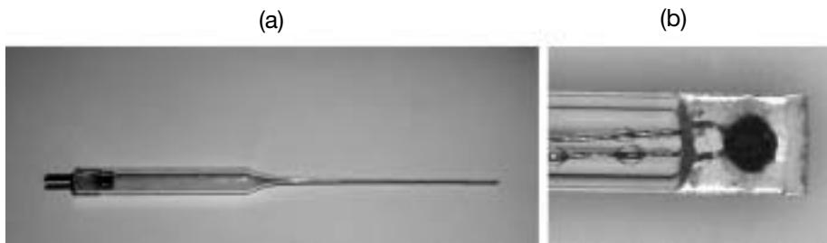
FIG. 1. (a) A thermistor pipette of the detector. (b) The small thermistor fixed in epoxy at the tip of the pipette. A thin glass rod seals this pipette version. In a different version (not shown) the thermistor is embedded in a massive glass rod 8 mm long.
