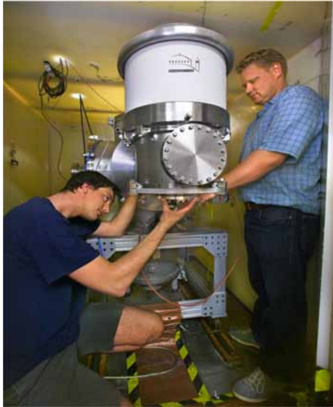
FIG. 35. Fabricated EUROSIA coaxial NG at the NG test stand at LBNL.
