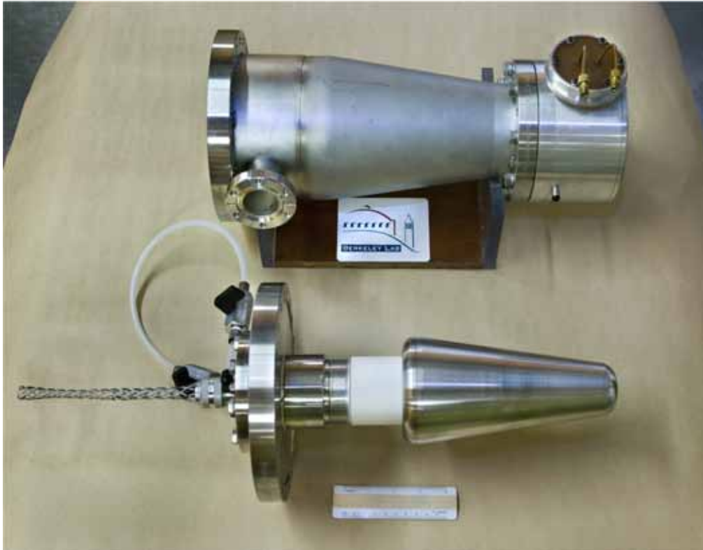
FIG. 30. The axial NG shown with target assembly separated (in the lower half of the picture) from the vacuum vessel and the ion source. The generator is 50 cm in length.
