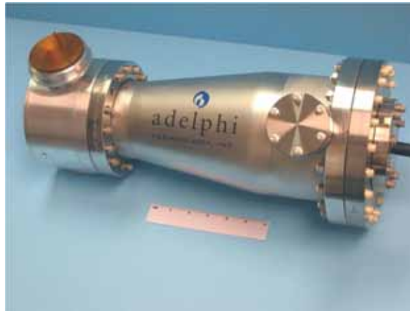
FIG. 17. An axial RFI NG. The components at high voltage potential are shielded by placing the entire accelerator structure and its components inside modified conflate stainless steel vacuum pipe. Not shown are the generator's required subsystems (i.e. vacuum, cooling and power supplies).
