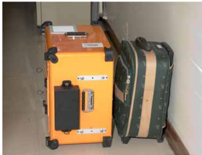
FIG. 10. The SODERN ULIS (Unattended Luggage Inspection System) system for inspection of suspicious object.
