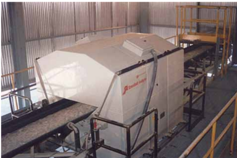
FIG. 8. Commercial Cross-Belt Analyzer, using the PGNAA technique for the cement industry.
