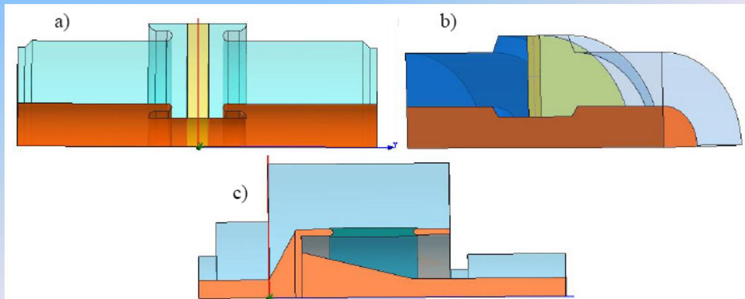
FIG. 4: Several window geometries: a) disk with chokes; b) disk without chokes; c) cylinder
