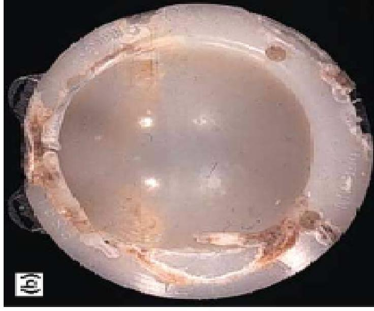
Fig. 2. Delamination associated with oxidation of: (a) UHMWPE tibial knee component and (b) UHMWPE acetabular hip component.
