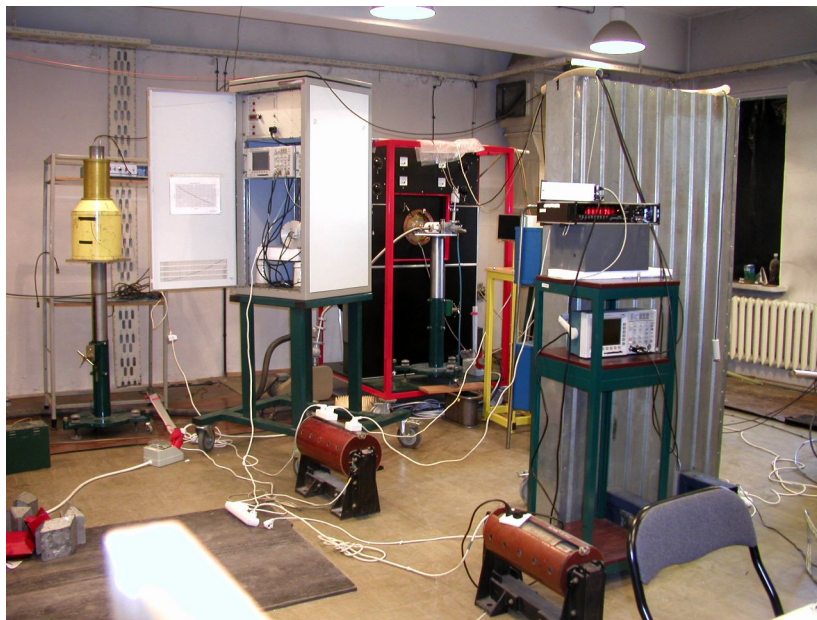
FIG. 1. PF-6 device (in the centre with red frame), its control unit behind the shadow shield on the right-hand side and the first fast photomultiplier-oscilloscope module on the left-hand side for time-of-flight neutron measurements
