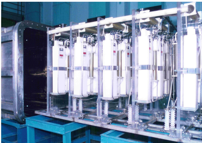
Fig.4 (a). Assembly of Marx Module of KALI-5000 Pulse Power System
