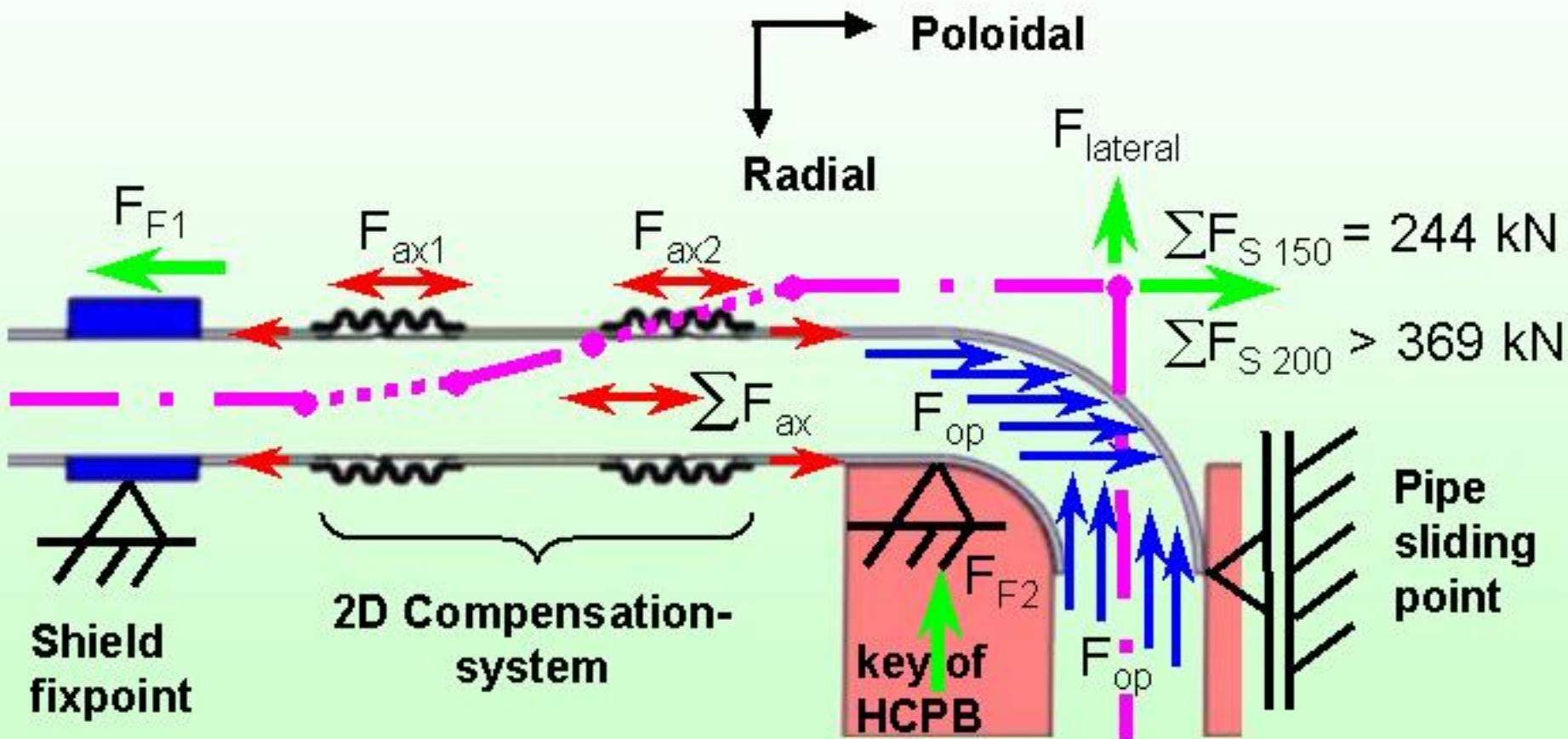
*Lateral and axial compensation bending process*
