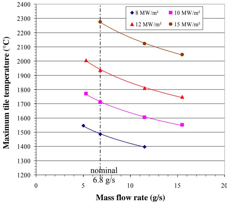
Fig. 4: Maximum tile temperature as a function of the He mass flow rate and heat flux, calculated for the reference HEMJ geometry (J1a).
