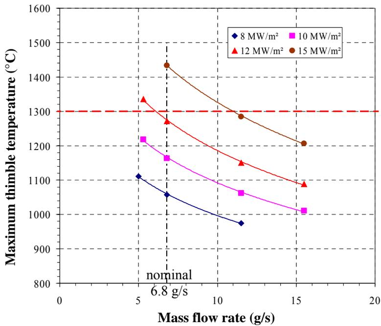
Fig. 5: Maximum thimble temperature as a function of the He mass flow rate and heat flux, calculated for the reference HEMJ geometry (J1a).
