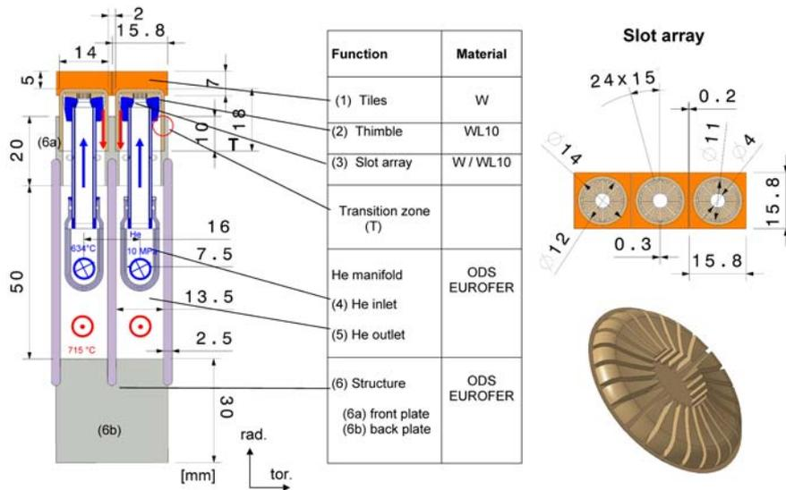
Fig. 2: He-cooled modular divertor design with slot array (HEMS).
