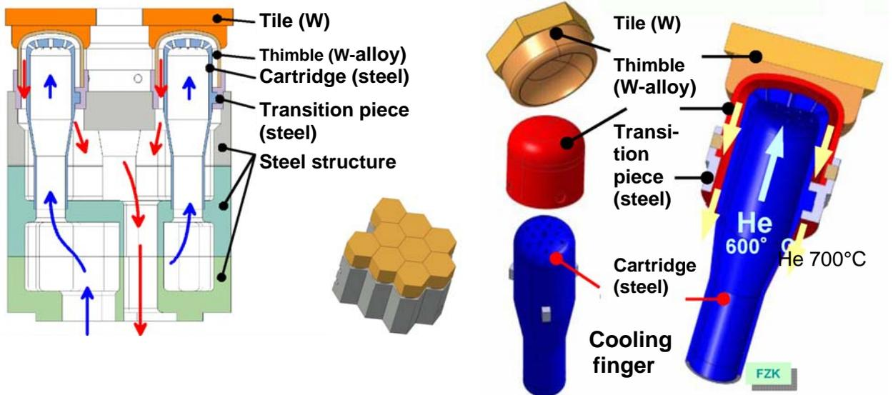
Fig. 3: He-cooled modular divertor with multiple-jet cooling (HEMJ).
