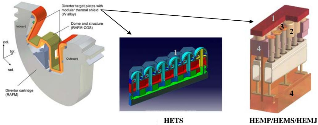
Fig. 1: Principle conceptual designs of divertor target cooling (1 W armour, 2 W thimble, 3 flow or jet flow promoter, 4 steel structure).
