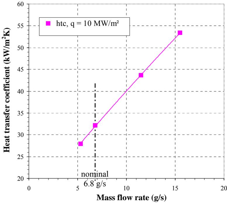
Fig. 6: Mean heat transfer coefficient (related to bulk temperature) as a function of the He mass flow rate, calculated for the reference HEMJ geometry (J1a),  $q = 10 \text{ MW/m}^2$ .
