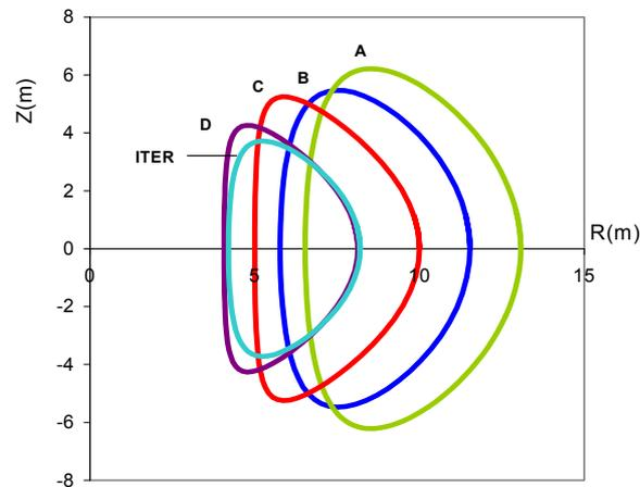
Fig. 1. The sizes and shapes of the plasmas in the four PPCS Models. For comparison, ITER is also shown: this is similar in size to Model D. The axes labels denote major radius ( $R$ ) and height ( $Z$ ).
