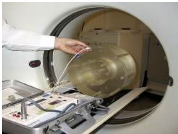
Measurement of dose in standard CTDI PMMA body phantom.
