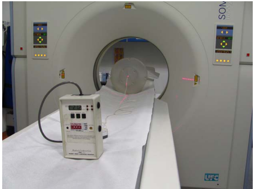
Typical set-up for clinical CT dosimetry, see also Chapter 9.6. of IAEA Human Health Series No. 19. (Courtesy of C. Hourdakis)
