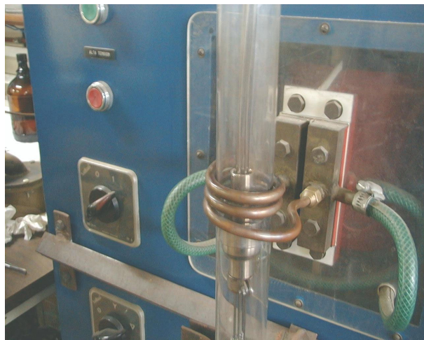
FIG. 6. Initial mounting for the welding.
