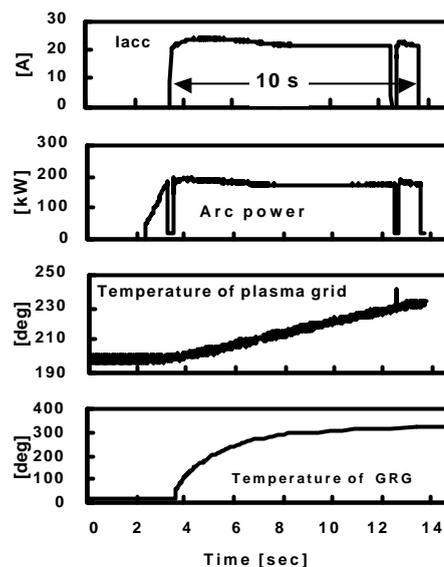
FIG.8 Time evolution of ion source parameter at 10 second injection
