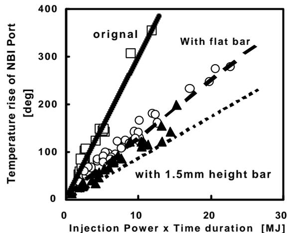
FIG.3 Temperature rise of the beam limiter at NBI port
