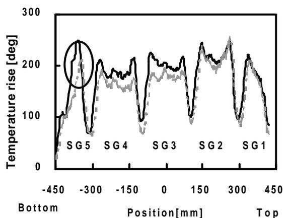
FIG.6 Longitudinal beam profile at 3.5m. Gray dotted line is uniform arc power and black line is enhance at bottom
