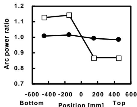
FIG.5 Arc power distribution by adjusting each filament voltage. Black circle is uniform and white square is enhanced at the bottom
