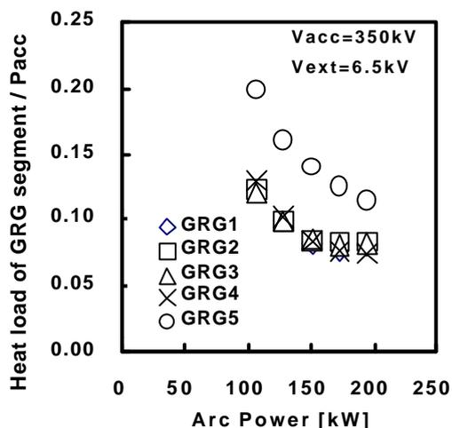
FIG.4 The heat load on GRG segments as a function of the arc power
