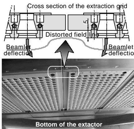
FIG.2 Grooves at the bottom of the extractor
