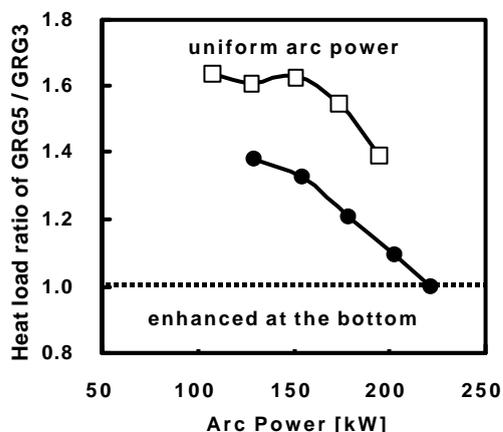
FIG. 7 The ratio of heat load on the segments between bottom and center. White square is for the uniform arc power and black circle is for enhanced at the bottom
