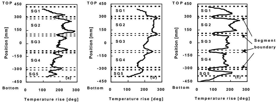
FIG.1 Longitudinal beam profile at 3.5m from ion source (a) original (b) with flat bar (c) with 1.5mm height bar
