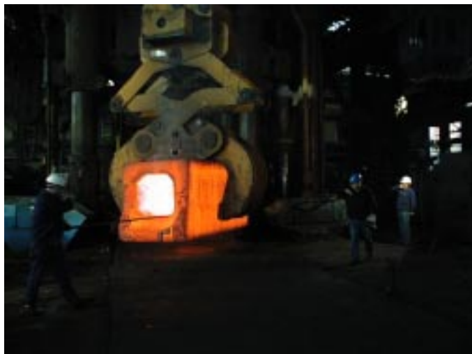
FIG. 11. Forging of inner leg curved section of TF coil case as hollow tube.
