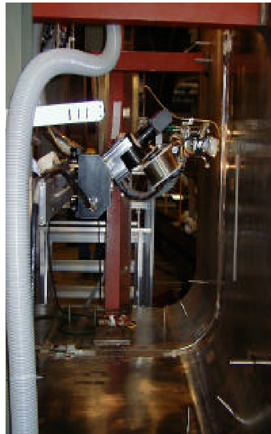
FIG. 3. The remotized welding tool.
