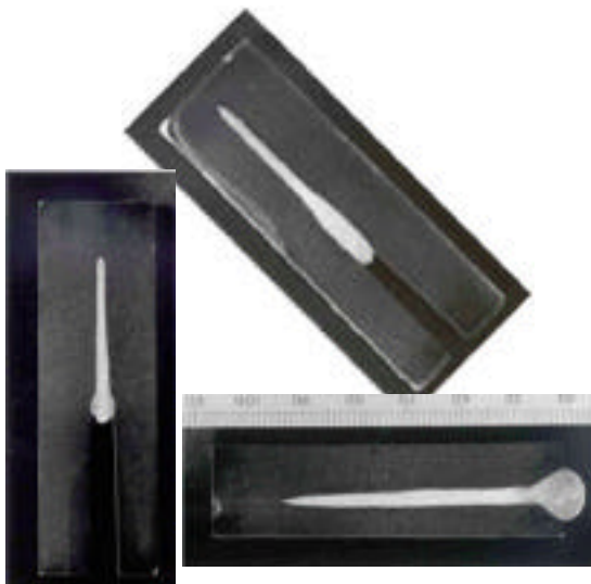
FIG. 4. RPEB welds at overhead, vertical plate and 45°.
