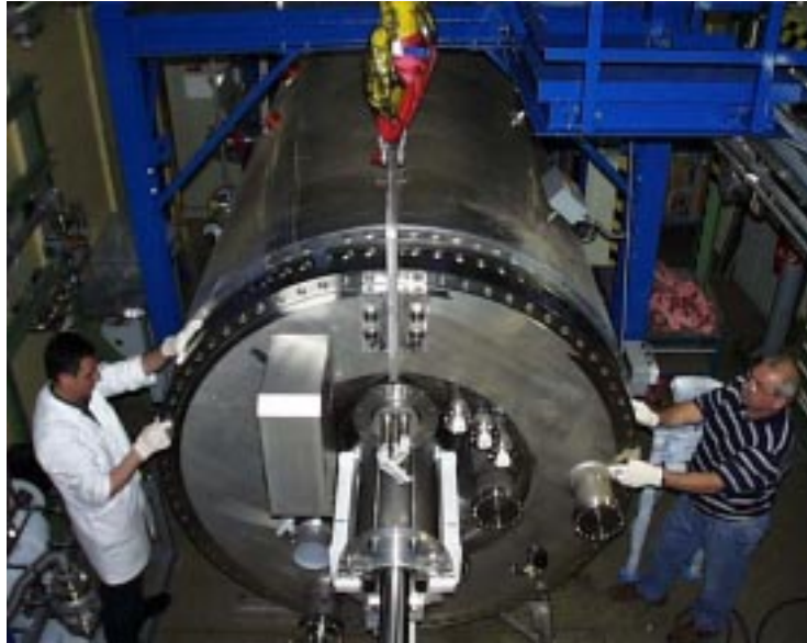
FIG 2. ITER Model Pump in Test Facility at FZK.
