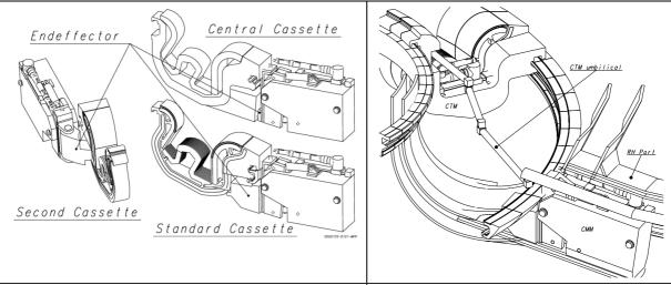
FIG. 3a: Cassette multifunctional mover (CMM) moves a divertor cassette radially through one of the 3 RH ports in a cantilevered way and is also able to place it sideways by one cassette width.
