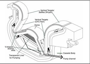
FIG. 1b: Divertor cassette showing the large openings in the dome support. Also shown is the transparent liner allowing pumping access from the private flux region.
