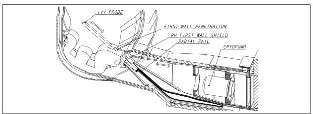
FIG. 4: IVV system allowing the deployment of up to 3 different  $\sim$  150 mm diameter probes through the upper part of a divertor cassette into the plasma chamber. Presently an IVV probe, a GDC probe and possibly a light manipulator (snake arm) are foreseen.
