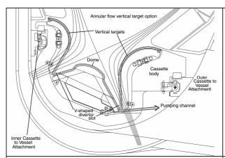
FIG. 1a: Cross-section through the divertor showing the V-shaped strike zones and the pumping path as well as the attachment to the toroidal rails.
