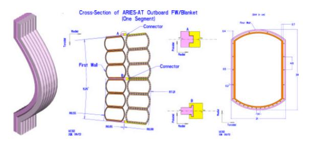
Fig 2. The ARIES-AT blanket module (1/2 of a blanket sector or 1/32 of the torus): A) Plan view, B) Cross section of the module, C) Cross section of a blanket "tube" showing the flow distribution insert.
