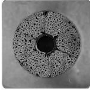
FIG. 1: Cross-section of SS-FSJS conductor.
