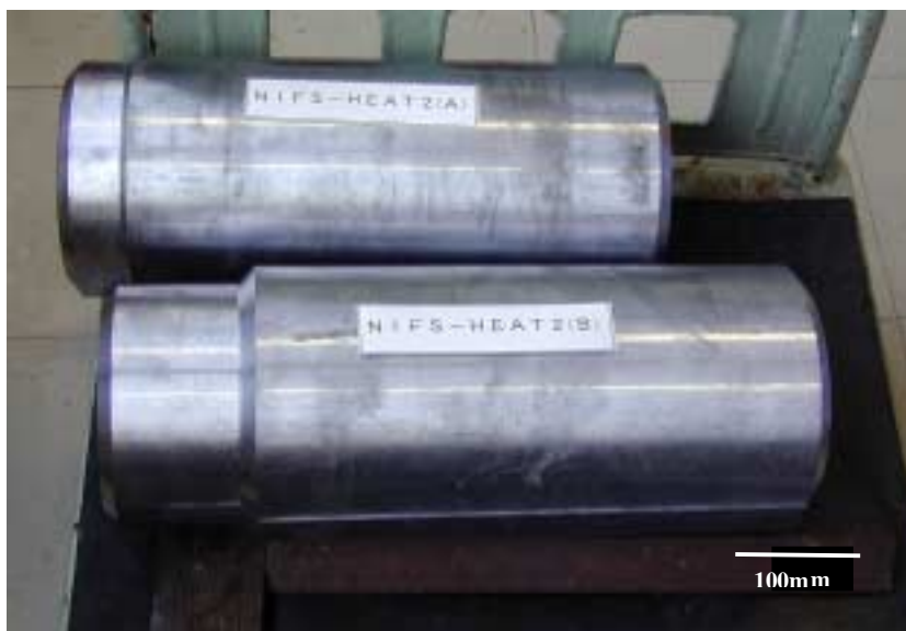
FIG.5. V-4Cr-4Ti ingots produced by the second fabrication after removing surfaces. NIFS-HEAT-2(A) (top) and NIFS-HEAT-2(B) (bottom).
