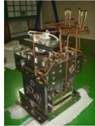
FIG. 6. Prototype of the magnet supporting post
