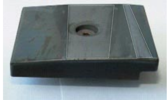
Figure 5: Tungsten coated tile at the end of the campaign. The erosion dominated areas are marked by a broken line.
