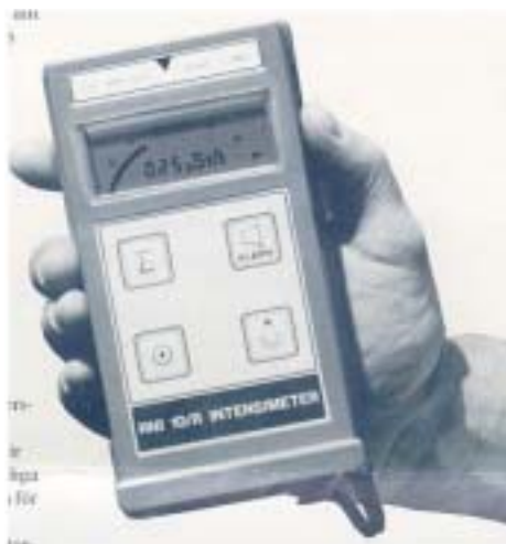
FIG. 1. The intensimeter (RNI 10/R) used by the Swedish customs.
