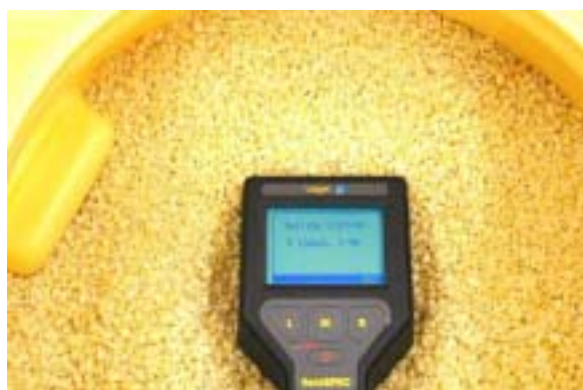
FIG. 6: Isotope identification test with fertiliser
