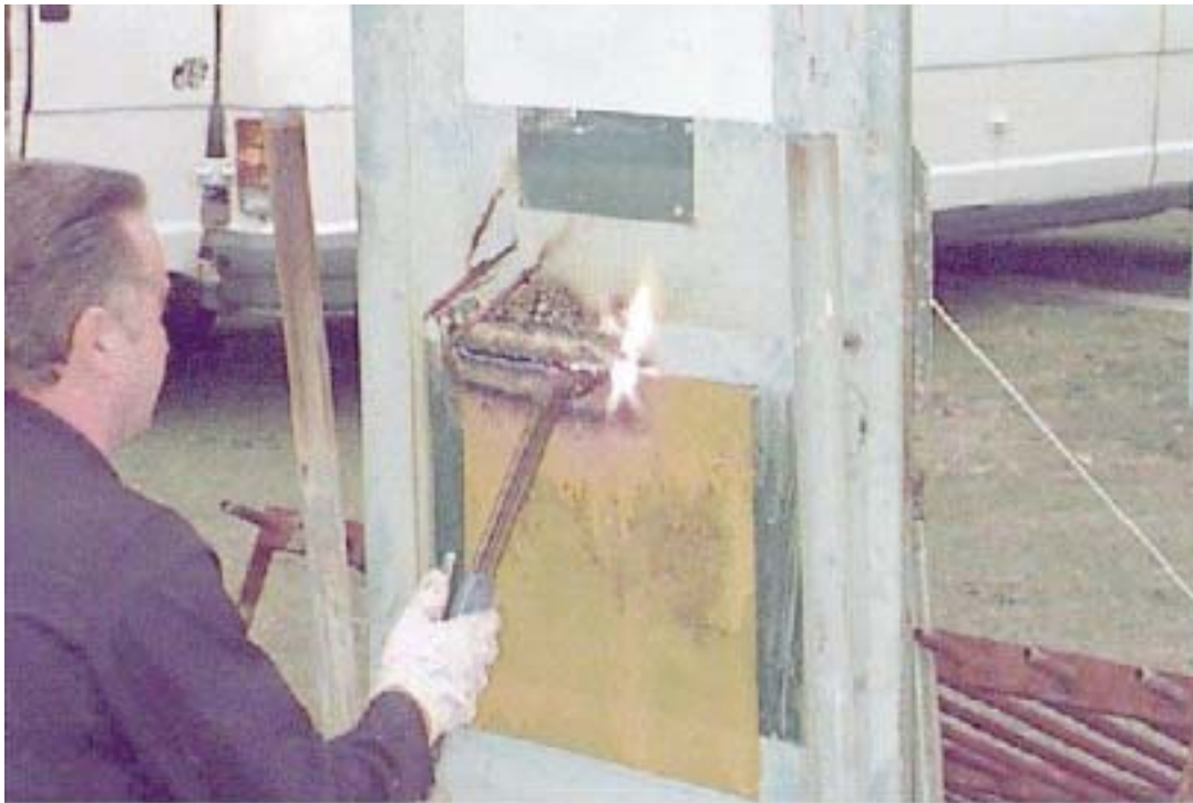
FIG. 2. Overcoming Test: Attack of a standard door consisting of 2 metal sheets (3 mm thick) Adversary: one aggressor. Techniques: drilling of a manhole (40 cm x 40 cm). Tool: soldering gun. Measured result: time to overcome.
