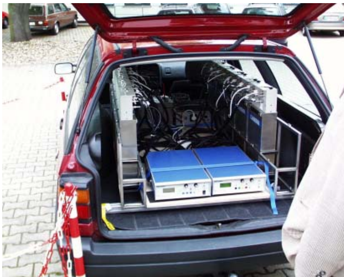
FIG. 1. Car with neutron slab counters and accessory electronics.
