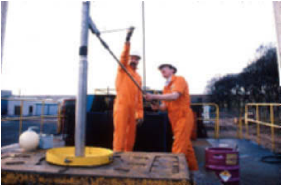
FIG. 11. Wireline engineers transferring radioactive sources to logging tools on the drill deck (courtesy: National Radiological Protection Board, UK).
