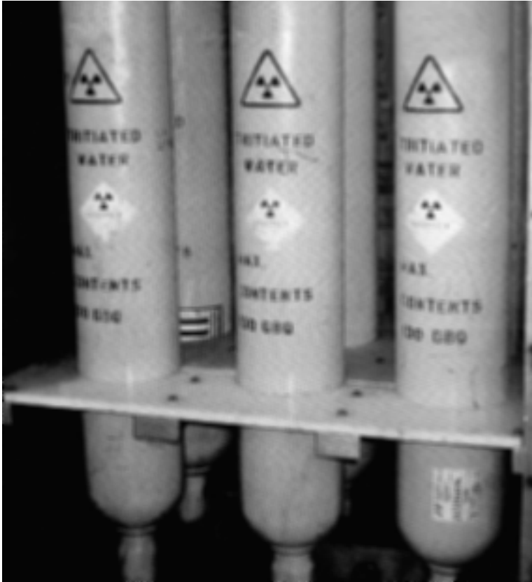
FIG. 20. Tritiated water for injection as a radioactive tracer (courtesy: Scotoil Group plc).
