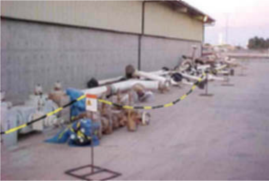
FIG. 27. Barrier designating a controlled area to restrict access to NORM-contaminated equipment stored outside a decontamination facility (courtesy: National Radiological Protection Board, UK).
