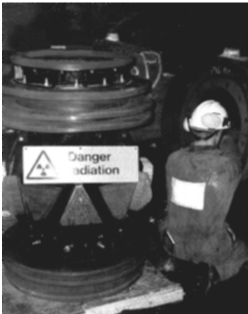
FIG. 7. Radioactive sealed sources incorporated in a pipeline pig (courtesy: Scotoil Group plc).
