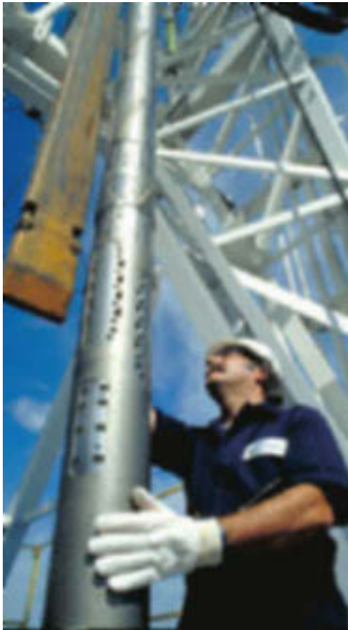
FIG. 8. Well logging tool string suspended by a derrick above an oil well (courtesy: Baker Hughes INTEQ).
