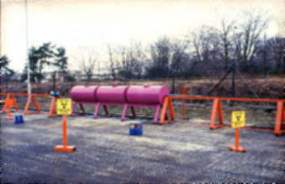
FIG. 13. Facilities to enable high dose rate radiation sources to be safely exposed during logging tool calibrations (courtesy: National Radiological Protection Board, UK).
