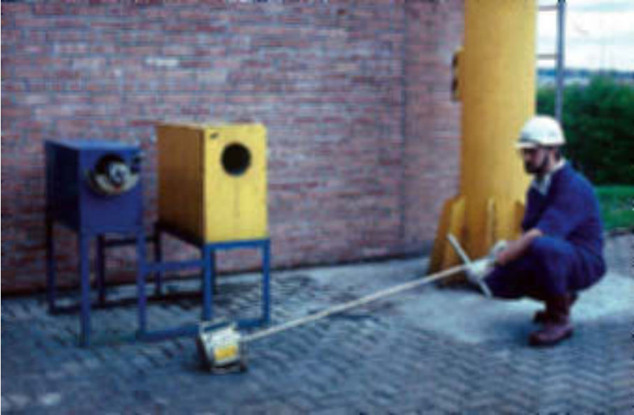
FIG. 12. Wireline engineer using a handling tool to transfer a radioactive source during a calibration procedure (courtesy: National Radiological Protection Board, UK).
