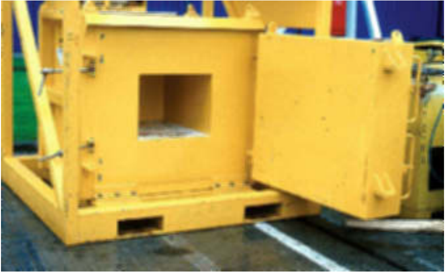
FIG. 10. Transport container used as a temporary store for well logging sources (courtesy: National Radiological Protection Board, UK).
