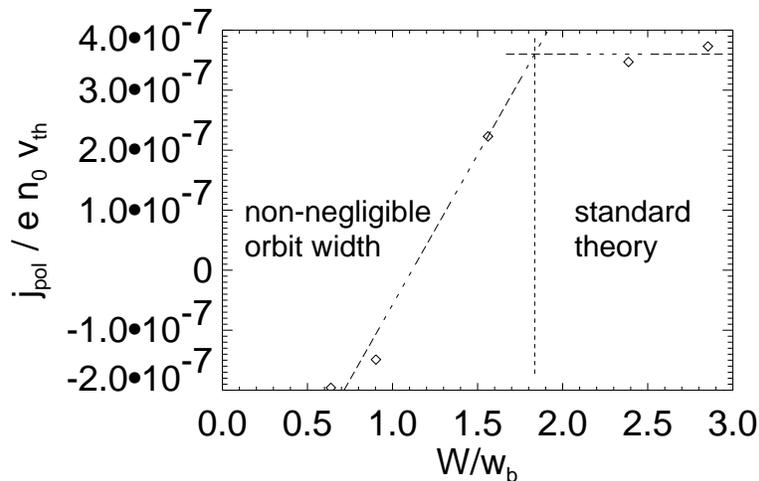
Figure 4: Polarisation current reduction for island widths  $W$  comparable to the ion banana width  $w_b$ .
