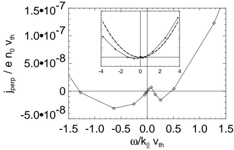
Figure 2: The perpendicular current  $j_{\perp}$  (normalised to  $en_0v_{th}$ ) as a function of the island rotation frequency  $\omega$  (normalised to the parallel streaming frequency  $k_{\parallel}v_{th}$ ). The dashed curve shows the estimate  $(\omega r/m)^2/r\omega_c v_{th}$ .
