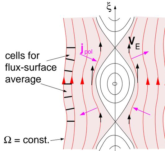
Figure 1: Polarisation current  $j_{\text{pol}}$  in the presence of a magnetic island.
