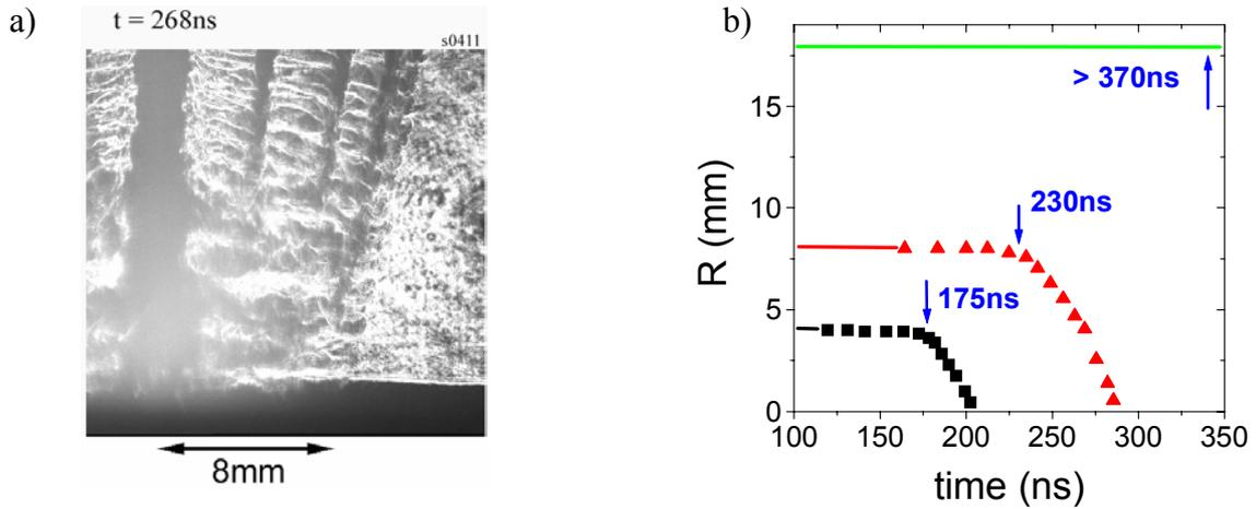
Fig. 1 Laser shadowgram of conical Al wire array (a) and implosion trajectories (b) measured from radial optical streaks for 32x15 $\mu$ m Al wire arrays of three different diameters.
