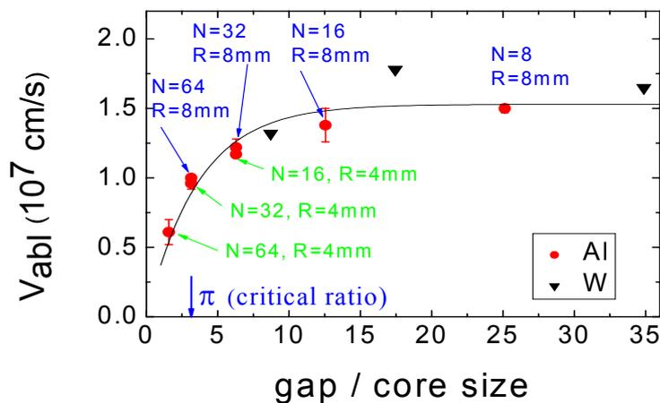
Fig. 2 Ablation velocity as a function of inter-wire separation for Al and W wire arrays. The inter-wire gaps are normalised on the core size measured by X-ray radiography. The line on the plot represents a fitting of the experimental data by a phenomenological formula  $V_{abl} = 1.5 \times 10^7 (1 - \exp(-x/3.4))$ , where  $V_{abl}$  is in cm/s and  $x = \text{gap/core size}$ .
