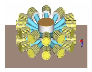
FIG. 4. LTD accelerator design (10 MA) [24].
