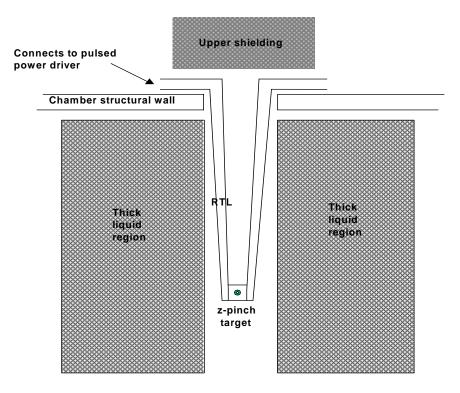
FIG. 2. The RTL (Recyclable Transmission Line) concept.
