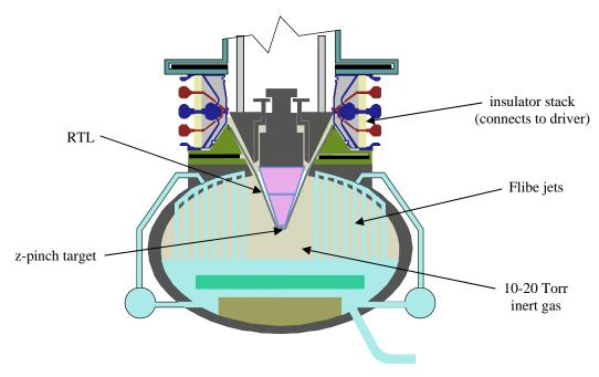
FIG. 6. Z-Pinch IFE chamber concept used in the ZP3 study [6,9].
