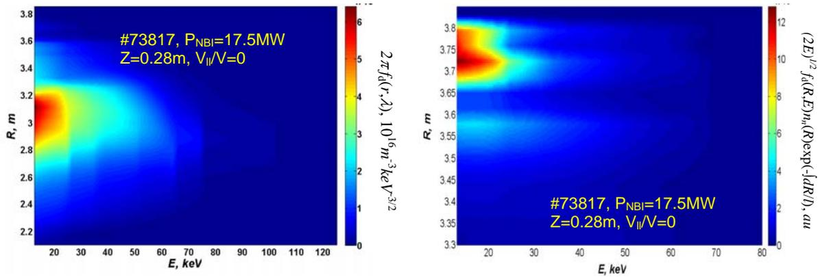
Fig. 3:  $R,E$  profiles of the distribution function of beam deuterons  $f_d(R, E, Z=Z_{LoS}, \xi=0)$  (left) and of the rate of  $D^0$  emission (right) detectable by NPA.
