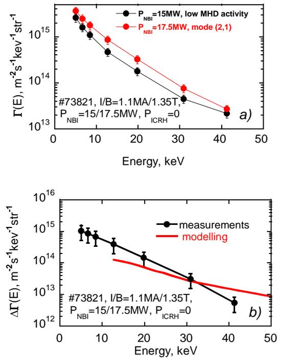
Fig. 10: (a) Measured  $D^0$  fluxes before and during MHD activity. (b) Modeled and measured increase of  $\Gamma(E)$  due to 2.5MW increase of  $P_{NBI}$  in shot 73821.
