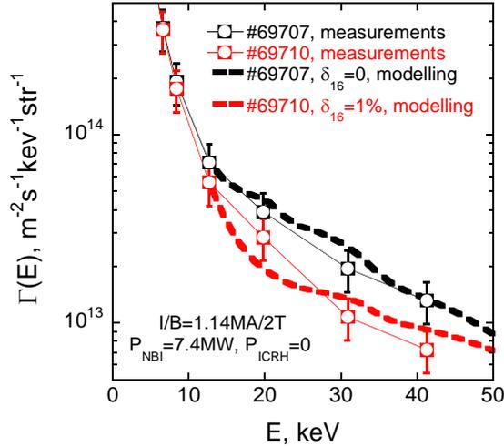
Fig. 6: Measured and modeled  $D^0$  fluxes in JET plasmas without (Pulse #69707,  $\delta_{16}=0$ ) and with (Pulse #69710,  $\delta_{16}=1\%$ )  $N=16$  TF ripple harmonic.
