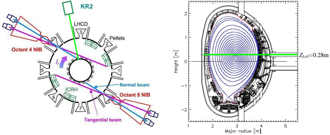
Fig. 1: Geometry of neutral beam injection and low-energy neutral particle analyser (KR2 NPA) on JET in toroidal (left) and poloidal cross-sections (right). The green line indicates the line-of-sight (LoS) of KR2.
