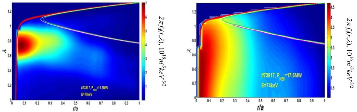
Fig. 2: Slices of the 3D COM distribution function of beam deuterons at energies  $E=74\text{keV}$  (left) and  $E=37\text{keV}$  (right) in the plane spanned by the normalized magnetic moment,  $\lambda = \mu B_0 / E$ , and the maximum radial orbit coordinate,  $r$ , for 17.5MW D-NBI in JET (Pulse 73817). The green lines represent the deuterons contributing to NPA signal.
