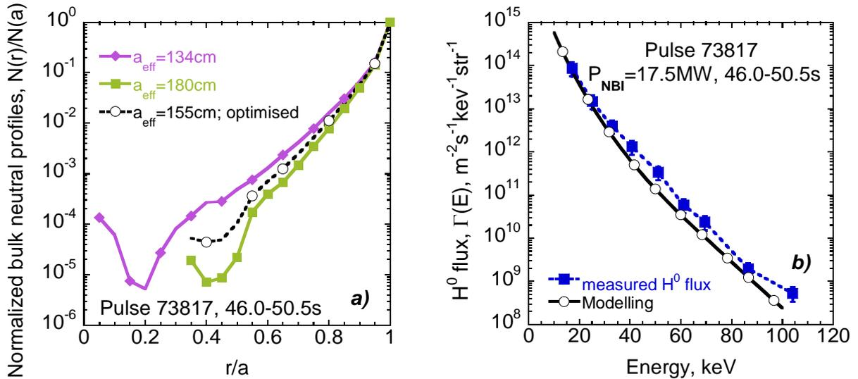
Fig. 5 Monte-Carlo modeled density profiles of bulk  $D^0$  neutrals (a). The optimised profile ( $a_{\text{eff}}=155\text{cm}$ ) in Fig.5a provides the best correspondence of the modeled  $H^0$  spectrum with the measured one in Fig.5b. This profile is used for calculation of the  $D^0$  spectra in Fig. 4.
