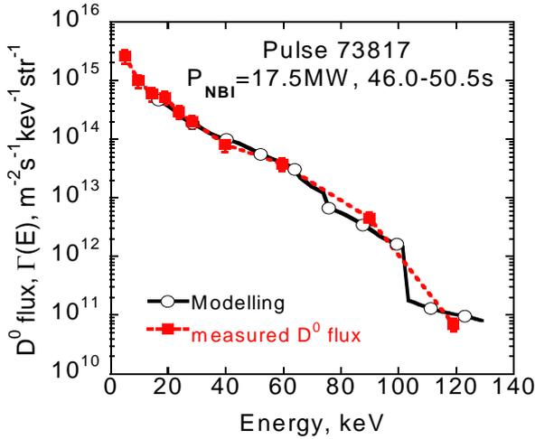
Fig. 4: Modeled and measured energy spectra of  $D^0$  fluxes emitted from NBI heated JET plasma (Pulse 73817).
