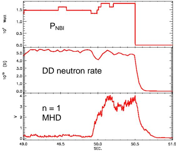
Fig. 8: Time traces of  $P_{NBI}$ , DD neutron rate and  $n=1$  MHD activity. Pulse 73821 ( $I/B = 1.1MA/1.35T$ )
