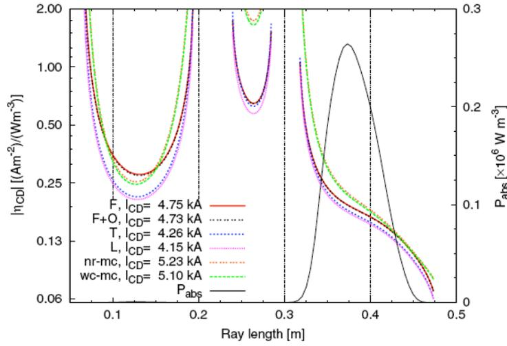
**Figure 3.** Values of the electron Bernstein current drive efficiency for several linear models, together with the absorbed power density profile. *F* is the Fisch model, *F+O* the Fisch model taking into account Ohkawa effect, i. e., particle trapping, *T* stands for Taguchi's model, *L* for the Lin-Liu model, while *wr-mc* and *nr-mc* denote weakly and non-relativistic momentum conservation models.
