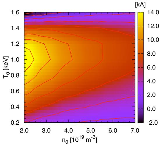
**Figure 5.** Total driven current by Bernstein waves in the TJ-II stellarator as a function of density and temperature. All the values are obtained by tracing 121 rays for plasma profiles like those shown in figure 2. The values of density and temperature correspond to the maximum values of the profiles.
