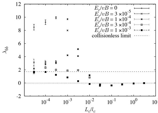
**Figure 1.** Monoenergetic coefficients for the bootstrap current calculated with NEO-MC for TJ-II, as a function of the mean free path, normalised by the thermal bounce path for the radial position given by the flux  $\psi = 0.25$ . The calculation is done for several electric fields.
