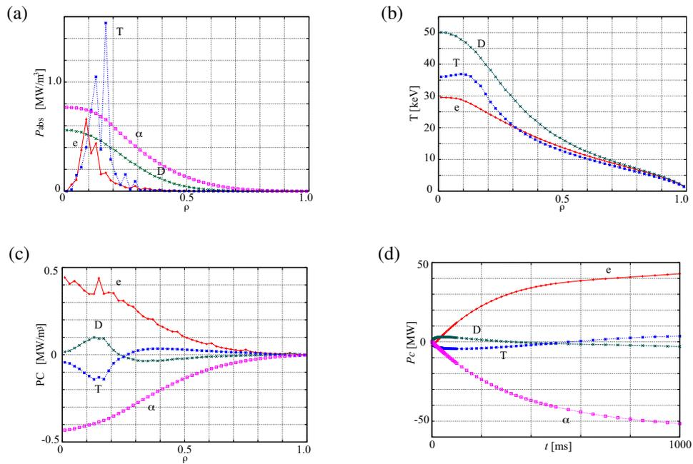
*Fig. 5. Radial profiles of (a) absorbed power density, (b) average kinetic energy, (c) collisionally transferred power density, and time evolution of collisional power transfer*
