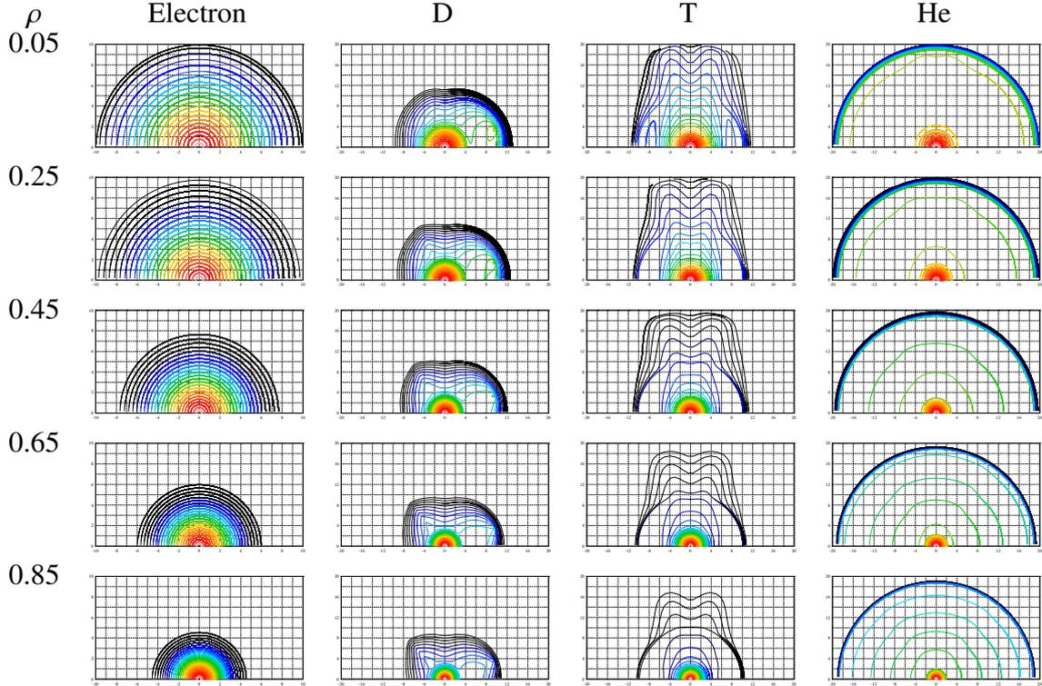
Fig. 4. Radial dependence of momentum distribution functions for electron, D, T, He.
