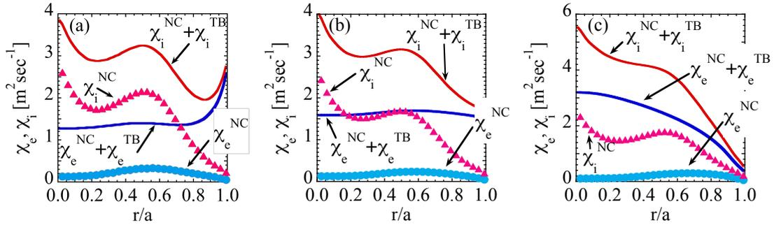
**FIG. 3.** The obtained thermal diffusivities of ion and electron with the turbulence (a) Alcator, (b) Bohm, and (c) gyro-Bohm model and the neoclassical transport.
