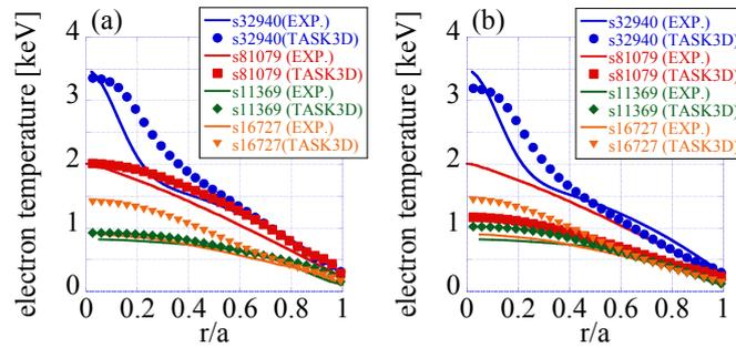
FIG. 4. Experimentally obtained electron temperature and temperature obtained by TASK3D with (a) gyro-Bohm model and (b) Alcator model.
