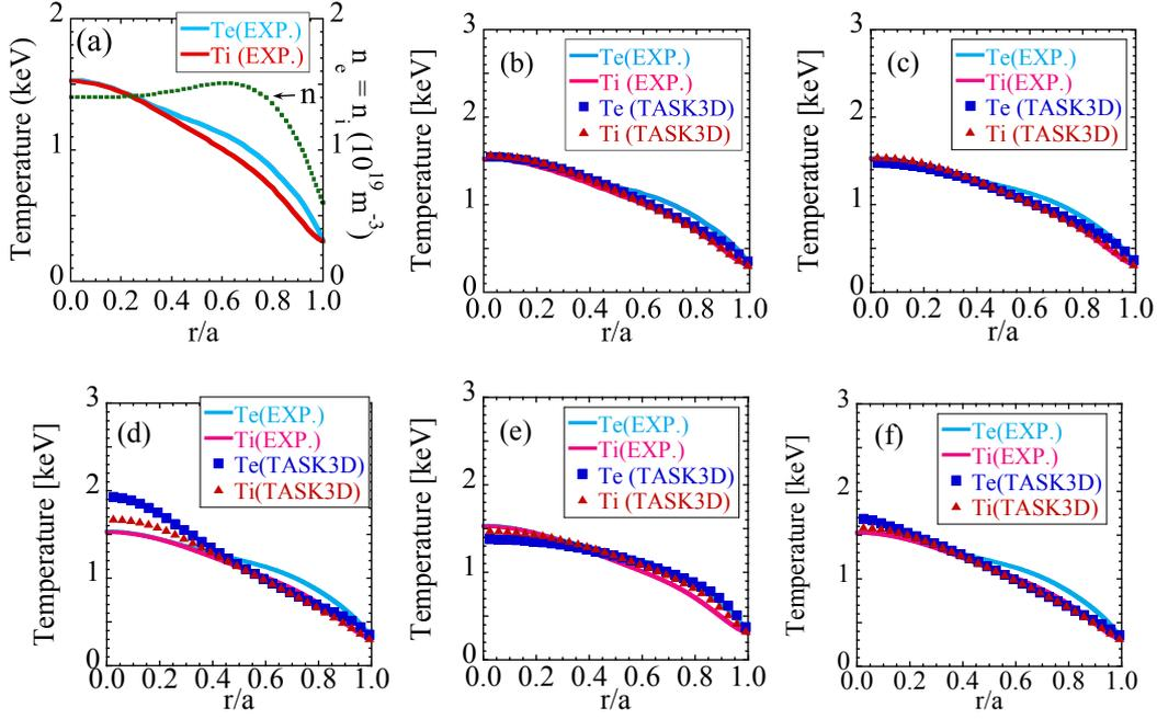
**FIG. 2.** (a) Initial profile of Te and Ti, and density (#88343). Comparison of the temperatures between experimental results and TASK3D results with (b) Alcator model, (c) Bohm model, (d) edge Bohm model, (e) gyro-Bohm model, and (f) gyro-Bohm multiplied by gradT model.
