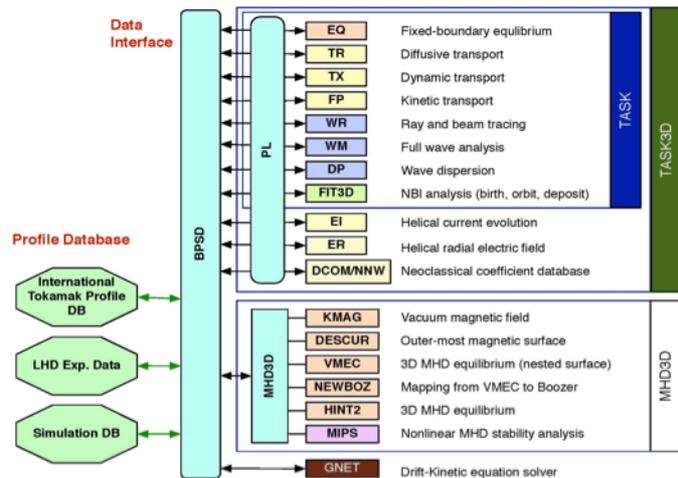
**FIG. 1.** Module structure of the core code of the integrated simulation code TASK with the extensions; TASK3D and MHD3D and GNET.
