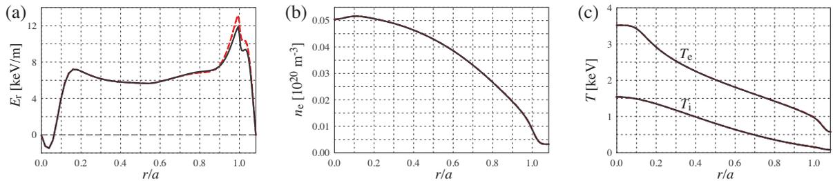
**FIG. 6.** Simulation results by TASK/TX for #32940, 2.003s; (a) radial profile of  $E_r$ , (b)  $n_e$ , (c)  $T_e$ ,  $T_i$ ;  $D_m=0$  (solid black line) and  $D_m=10^9$  m (dashed red).
