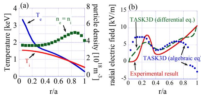
FIG. 5. (a) experimental profiles of  $T_e$ ,  $T_i$  and  $n$ , (b) experimental result of  $E_r$  (line) and simulation result solved by the algebraic equation (symbols) and by the differential equation (dashed line).
