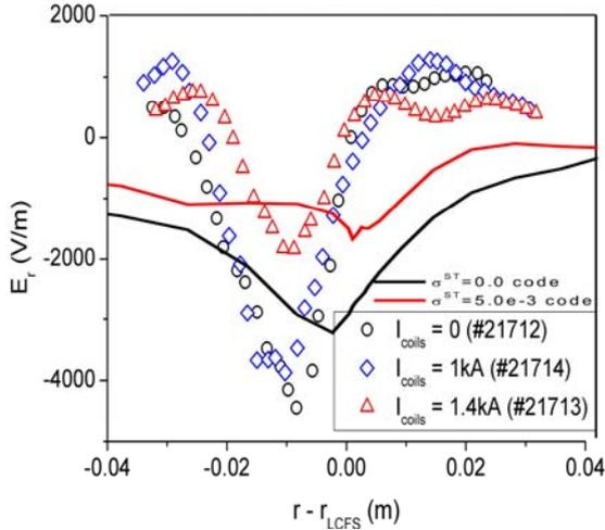
FIG.3. Comparison of experimental and simulated radial electric field profiles at the outer midplane for L-mode shots with and without RMP.
