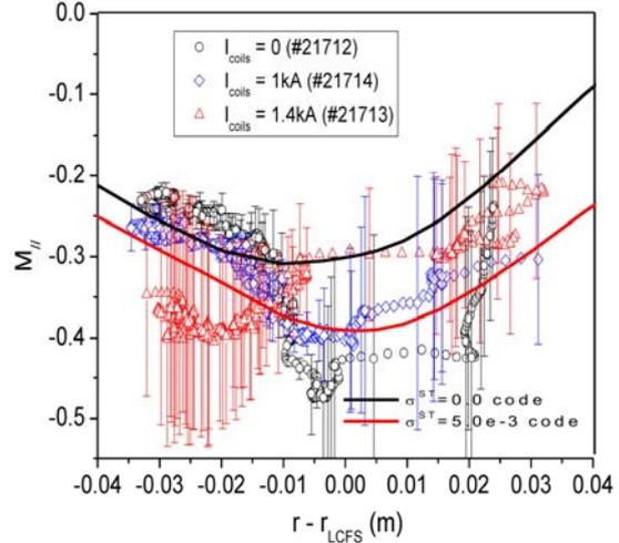
FIG.4. Comparison of experimental and simulated parallel Mach numbers at the outer midplane for L-mode shots with and without RMP.
