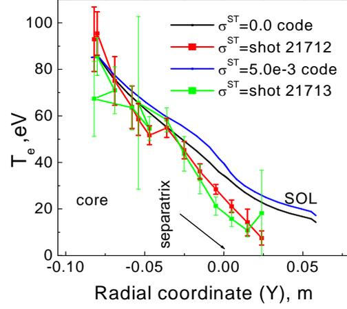
FIG.2. Electron temperature profile at the outer midplane for L-mode shot No21712 (without RMP) and shot No21713 (with RMP).
