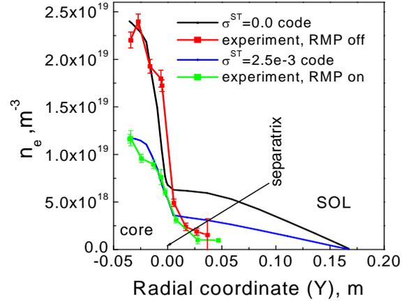
FIG. 6. Electron density profile at the outer mid-plane with and without RMP for H-mode shots №20387 and №20381.
