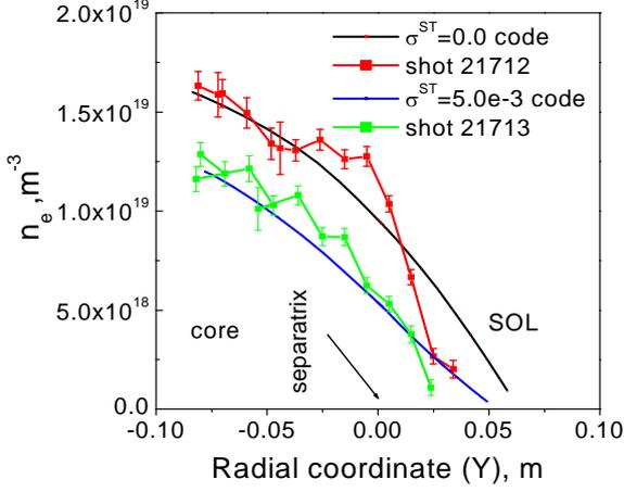
FIG.1. Electron density profile at the outer midplane for L-mode shot No21712 (without RMP) and shot No21713 (with RMP).
