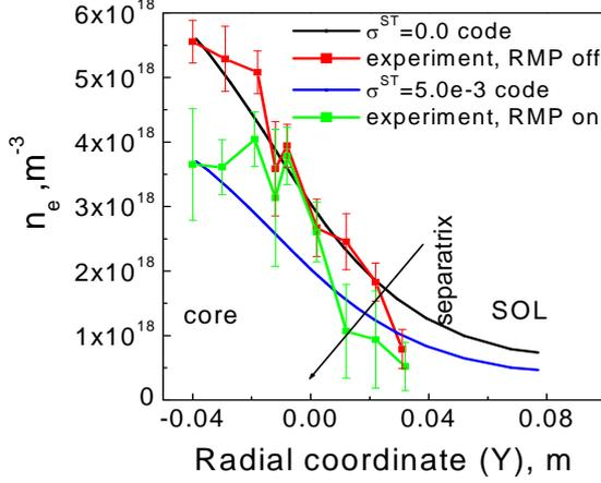
FIG. 5. Electron density profile at the outer mid-plane with and without RMP for low density L-mode shots №20449 and №20451.
