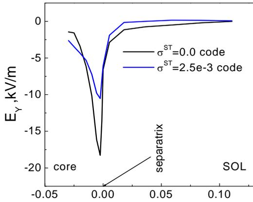
FIG. 7. Simulated radial electric fields at the outer mid-plane with and without RMP for H-mode shots №20387 and №20381.
