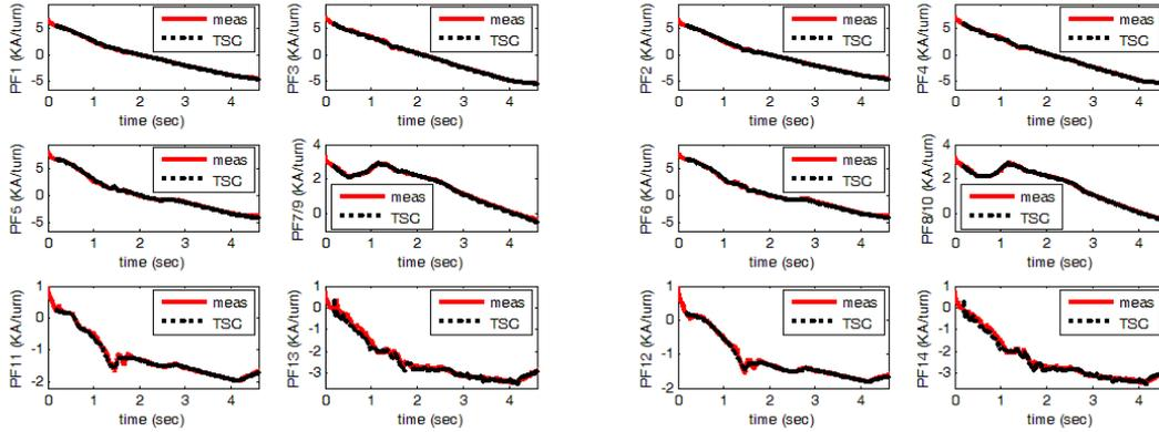
FIG. 4. Shot 17126 PF current (KA/turn) versus time (sec). (left) PF coils with the odd number, (right) PF coils with even number. PF7 and PF9, PF8 and PF10 connected together, respectively. In the figure, the measurements are shown by red line and the TSC simulated data by black dot line.
