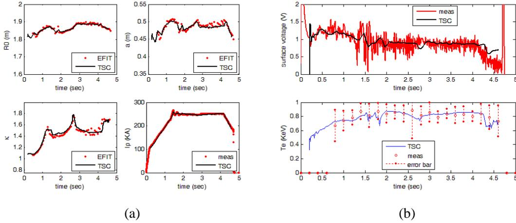
FIG. 5. Shot 17126. (a) The major radius (top left), the minor radius (top right), the elongation (bottom left) and plasma current (bottom right) versus time. (b) surface voltage (top): TSC simulated data (black line) fit experimentally measured values (red line) well, and electron temperature (bottom) at (1.90 m, 0.0),  $T_e$  trajectory at this point simulated by TSC (blue line) follows the soft x-ray measurements (red circular) well considering the measurement error bar (dot line).
