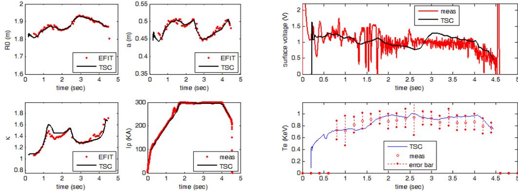
FIG. 7. Shot 17127. (a) The major radius (top left), the minor radius (top right), the elongation (bottom left) and plasma current (bottom right) versus time. TSC predicted data (black line) fit experimentally measured values (red line) well due to TSC control system. (b) surface voltage (top):and electron temperature (bottom) at (1.90 m, 0.0) (bottom).
