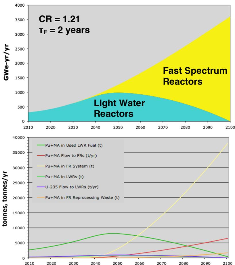
FIG. 2a, b. Power production and stocks and flows of Pu + MA and  $^{235}\text{U}$  for fast-spectrum reactors.
