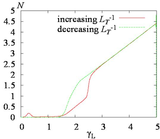
Fig. 3. Plots of evolution of turbulence intensity  $N$  versus temperature gradient ( $\gamma_L$ ) in cases with induced ramp up/down of  $L_T^{-1}$ .
