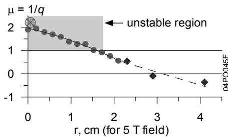
**Fig.3** Rotary transformation factor at  $T = 3.5 \cdot 10^{-6}$  s after start of the REB injection. Black circles - X-ray footprint, cross – current density on the exit, diamonds – current measurements on the entrance of the system.
