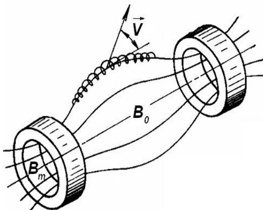
**Figure 1** A scheme of magnetic mirror
