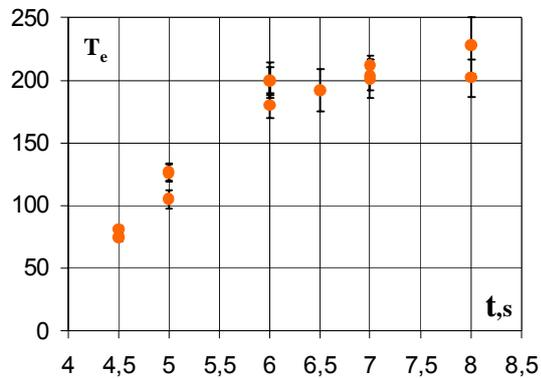
**Fig.5** Temperature dependence on time at NB injection power  $P_{inj} = 6$  MW
