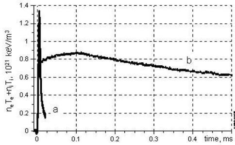
**Fig.2** Temporal behavior of plasma pressure after REB injection
