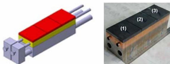
*FIG. 3. Blanket FW mock-up design and fabrication for prequalification tests.*
