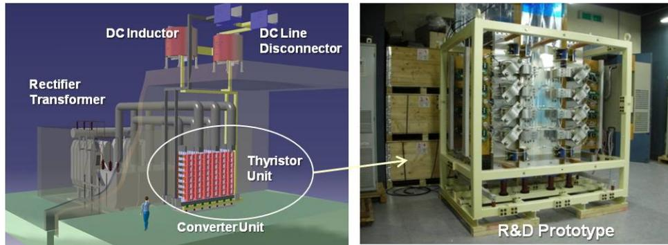
FIG. 7. The Proto-type system of the ITER AC/DC converter.
