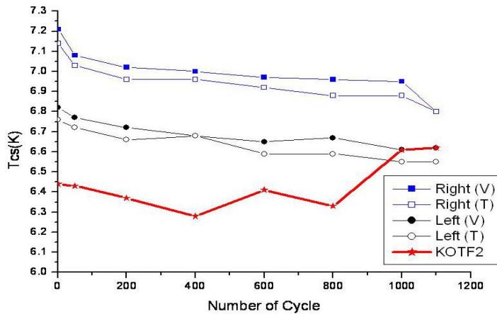
FIG. 2. Conductor Performance Qualification Sample test results at SULTAN.
