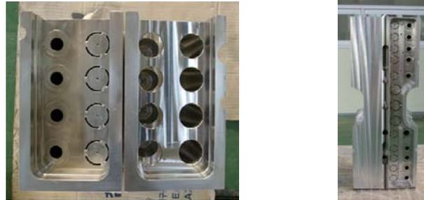
FIG. 4. Blanket shield block mock-ups.
