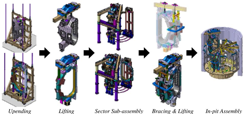
*FIG. 6. Overall configuration of the sector sub-assembly and in-pit tools.*
