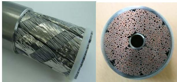
FIG. 1. Dummy CICC Sample.
