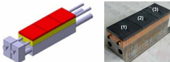
FIG. 3. Blanket FW mock-up design and fabrication for prequalification tests.
