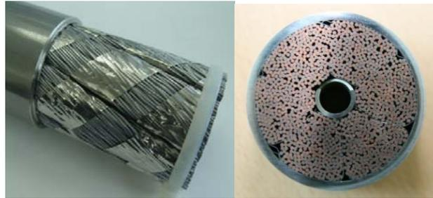
FIG. 1. Dummy CICC Sample.
