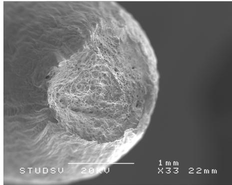
FIG. 4. SEM image of the fracture surface of a 316L(N)-IG exposed at 200 °C, in ultrapure water containing 1000 ppb H<sub>2</sub>O<sub>2</sub> and 100 ppb Cu<sup>2+</sup>.
