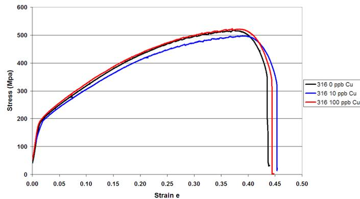
FIG. 2. Stress-strain curves for 316L(N)-IG specimens exposed to different levels of soluble  $\text{Cu}^{2+}$ .
