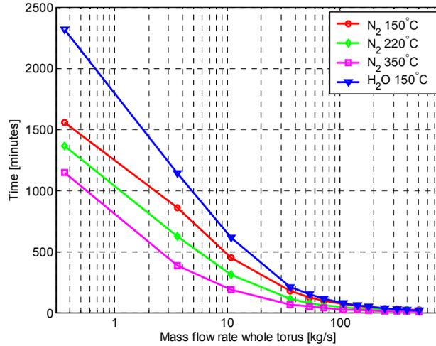
FIG. 8. Drying time when the initial water and structure temperature is 110 °C.
