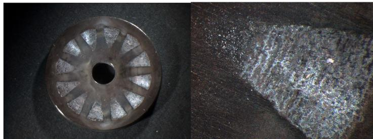
FIG. 5. Photographs of minor crevice corrosion attacks on a SS 430 specimen after 15 drying cycles using superheated steam.
