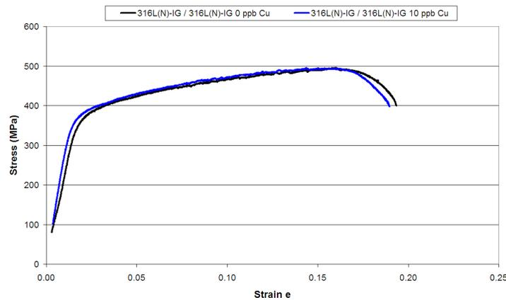
FIG. 3. Stress-strain curves for TIG narrow gap welded 316L(N)-IG specimens exposed to different levels of soluble  $\text{Cu}^{2+}$ .
