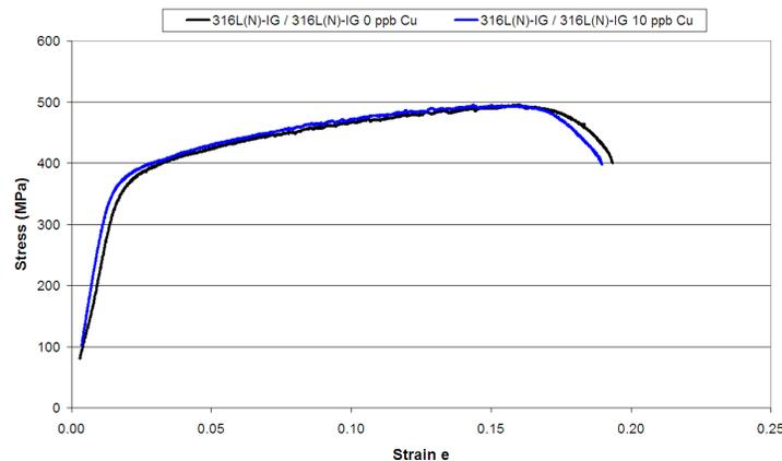
FIG. 3. Stress-strain curves for TIG narrow gap welded 316L(N)-IG specimens exposed to different levels of soluble  $\text{Cu}^{2+}$ .
