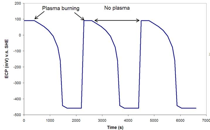
FIG. 1. The change in ECP of stainless steel piping as a function of the consecutive periods of plasma burning 400 s followed by dwell periods of 1800 s.
