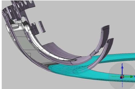
FIG. 6. 3D model of the water remaining at the bottom of the Vacuum Vessel after draining.
