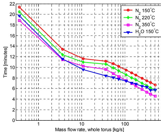
FIG. 7. Drying time when the initial water and structure temperature is 200 °C.
