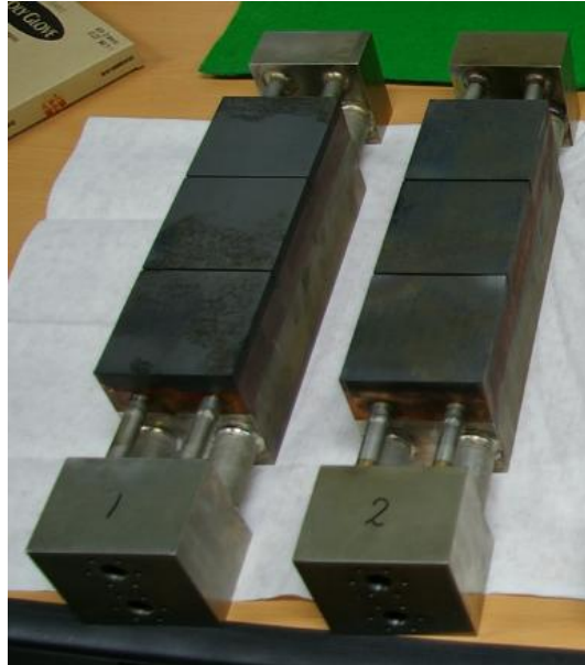
FIG. 2. Be/Cu/SS mock-ups for the HHF test in TESFEY.
