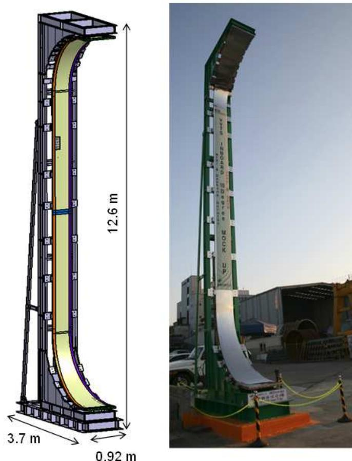
*FIG. 8. Assembly of Full-scale mock-up of Inboard 10 degree section of VVTS.*
