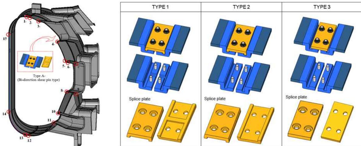
FIG.4 Design of the in-pit joint for ITER thermal shield.
