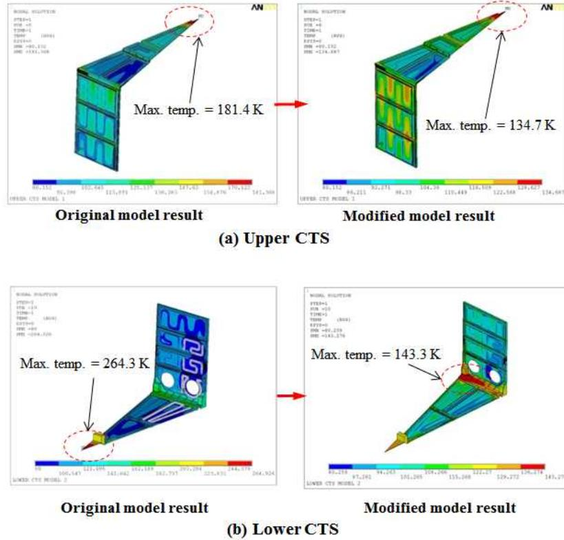
FIG. 3. Results of thermal analysis for upper and lower CTS.
