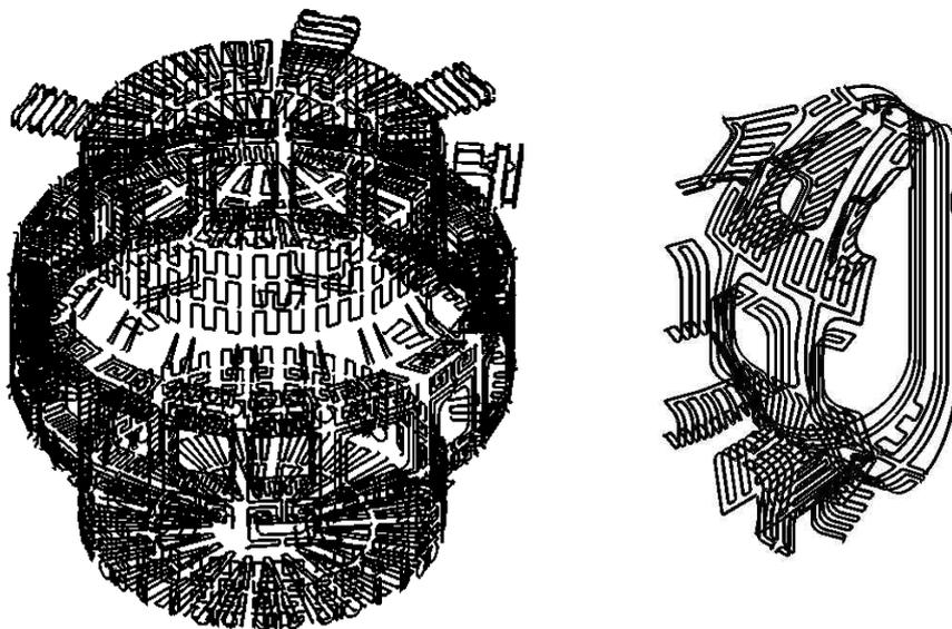
FIG. 2. Design of the cooling line for ITER thermal shield.
