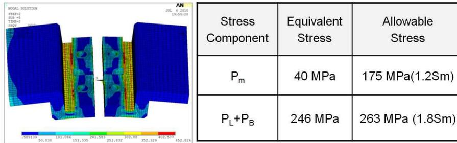
FIG.5 Structural analysis result of in-pit joint for ITER thermal shield.
