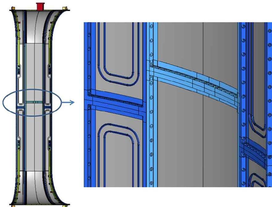
FIG. 6. Design of the bisecting joint for VVTS inboard 10 degree.
