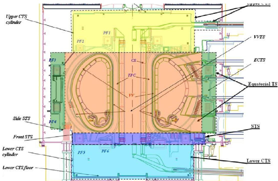
FIG. 1. Configuration of ITER thermal shield.
