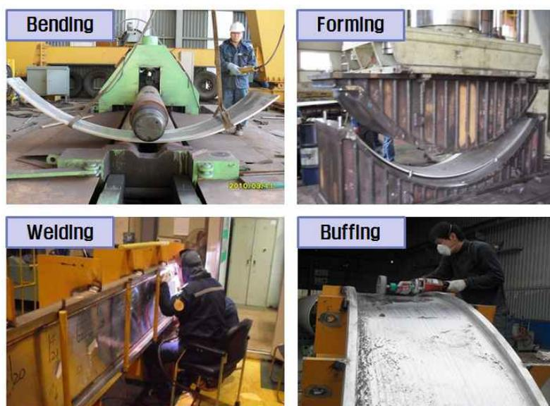
*FIG. 7. Manufacturing process of the mock-up.*
