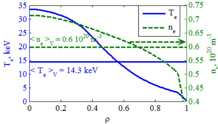
FIG. 2. Electron temperature and density profiles for the steady-state regime of ITER operation [9], used for comparison of EC power loss profile predictions (see FIG. 4).
