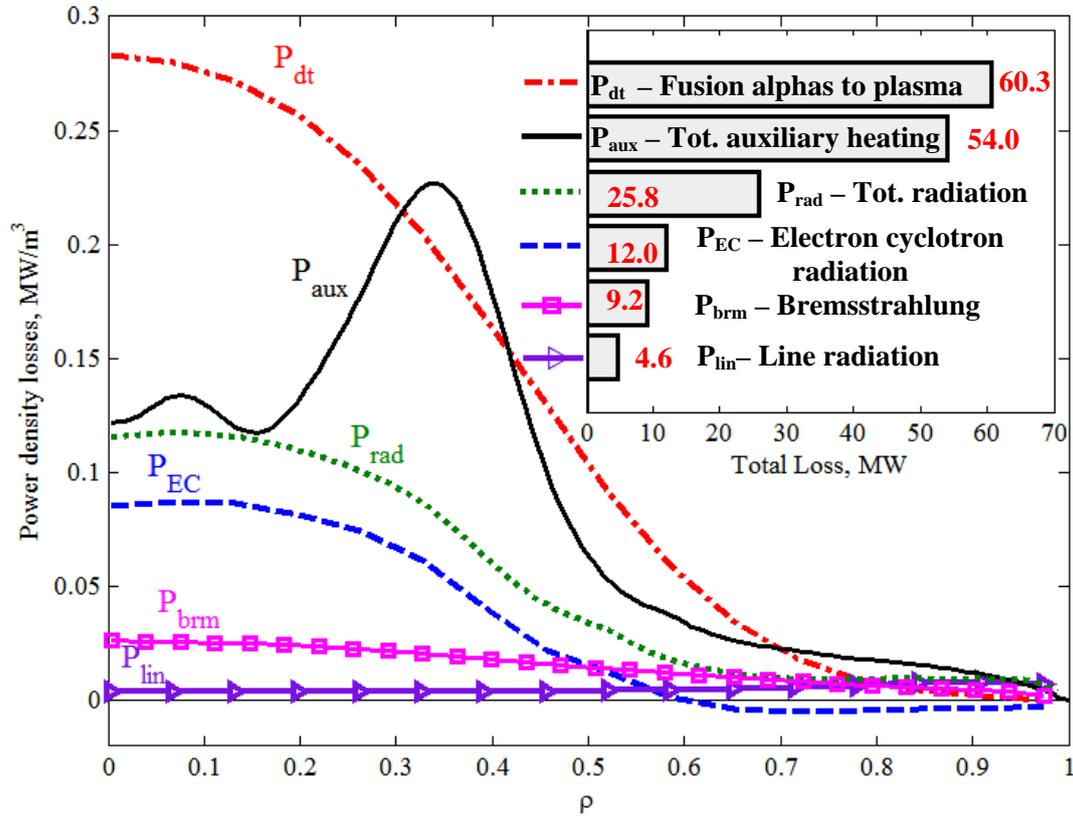
FIG. 5. Comparison of components of the local energy balance for scenario [9] with  $T_e$  and  $n_e$  profiles from FIG. 2. Inset: comparison of total power losses.
