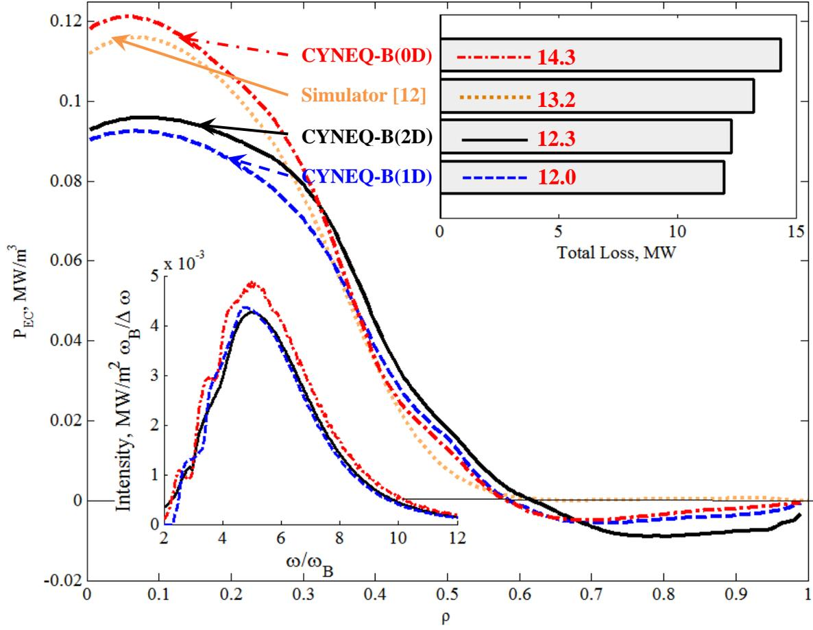
FIG. 4. Profiles of EC power density losses,  $P_{EC}(\rho)$ , predicted by CYNEQ, for three different cases of magnetic field approximation for self-consistent 1.5D transport simulations [9] for temperature and density profiles displayed in FIG. 2. Volume-integrated total outgoing ECR losses are shown in the legend. Inset: respective intensities of outgoing radiation as a function of frequency normalized to fundamental gyrofrequency for vacuum toroidal field on the vessel's axis.
