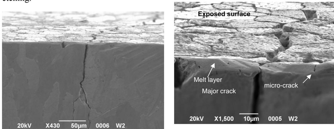
*Fig.3. Cross-section of the deformed W target preheated at 200 °C and exposed to 10 pulses of 0.75 MJ/m<sup>2</sup>*
