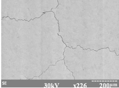
*Fig.2. Major cracks on W surface after 5 pulses of 0.45 MJ/m<sup>2</sup>. T<sub>0</sub>=200 °C*
