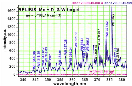
Fig.5. Spectral lines recorded within the RPI-IBIS experiment (with and without W-target) in spectral range (340-380 nm).
