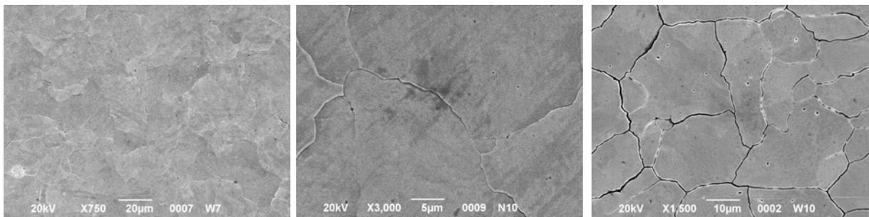
*Fig.4. W surface after 5 pulses of 0.75 MJ/m<sup>2</sup>, at T<sub>0</sub>=400 °C; after a single pulse, and after 5 pulses of 0.75 MJ/m<sup>2</sup>, at T<sub>0</sub>=600 °C.*
