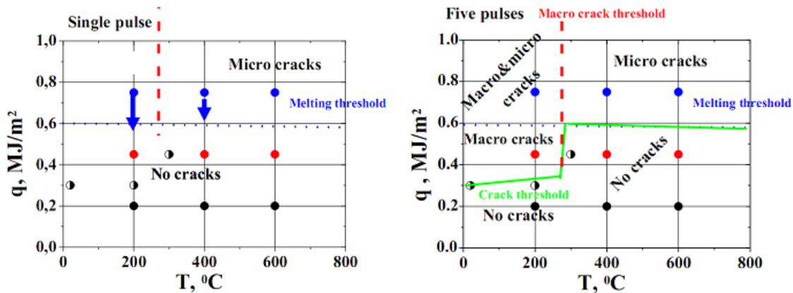
Fig.1. Cracking thresholds diagrams for ITER reference W grade: after a single pulse (a) and after 5 (b) QSPA plasma pulses
