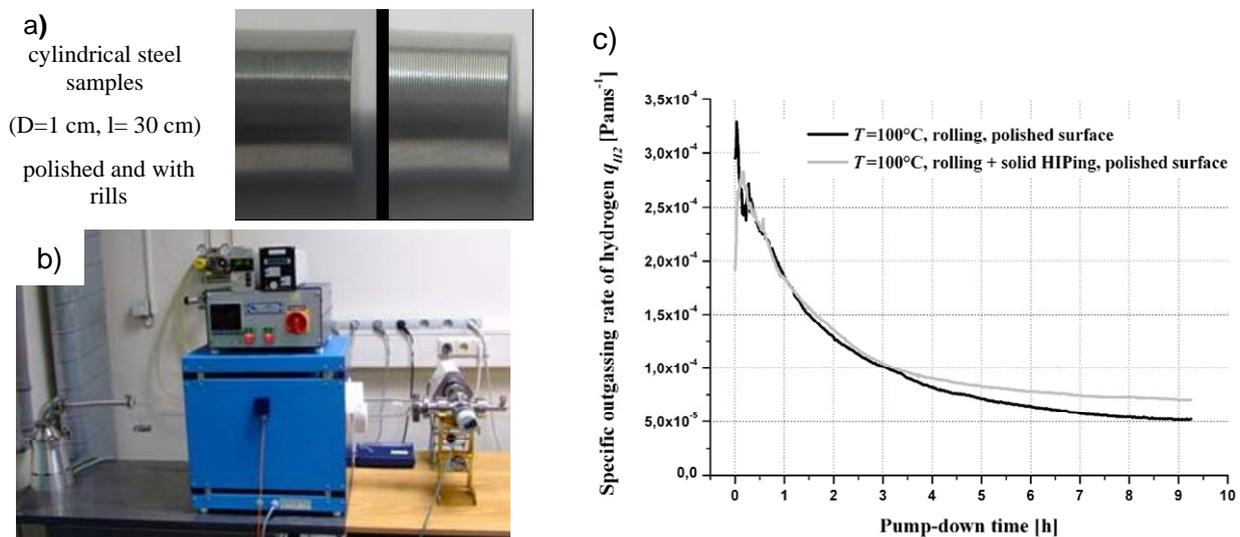
*FIG. 8. a) Typical samples, b) experimental set-up c) effect of HIP on the specific outgassing rate.*
