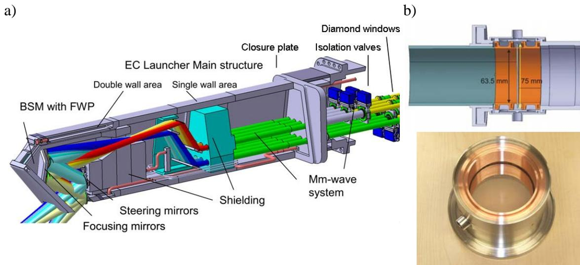
*FIG. 1. a) Overview: main components of the ECRH Upper Launcher, b) Diamond torus window concept and prototype.*
