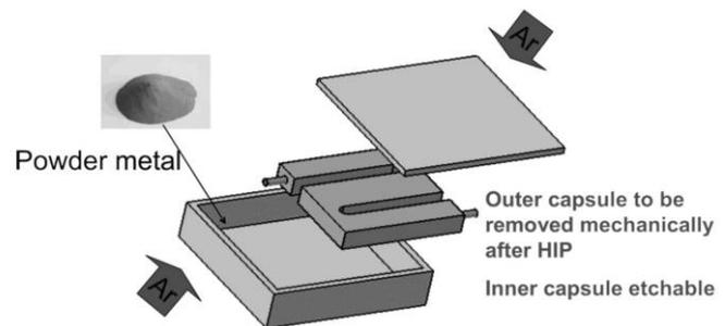
FIG. 5. Schematic layout of the test samples for a) diffusion welding and b) powder metal sintering by HIP.
