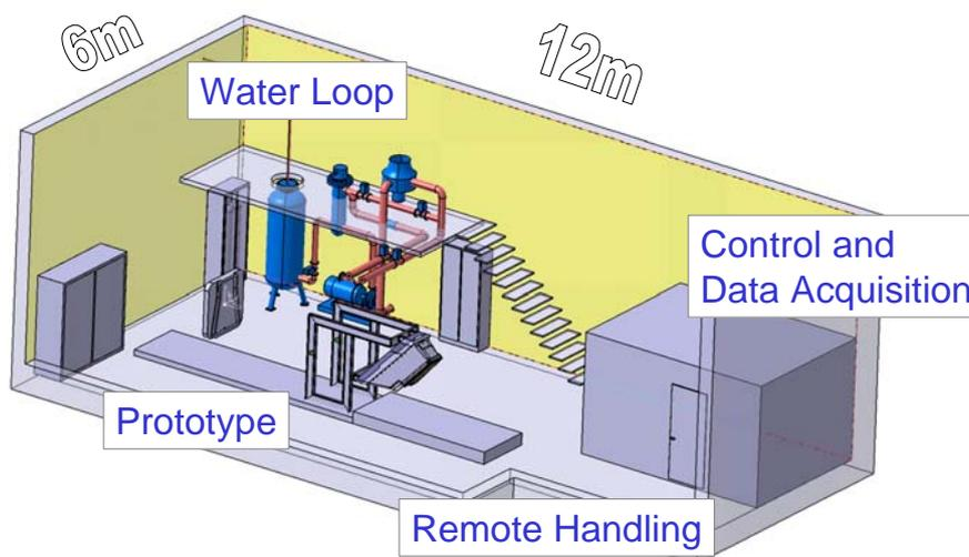
FIG. 2. Schematic configuration of the Launcher Handling and Test facility (LHT).
