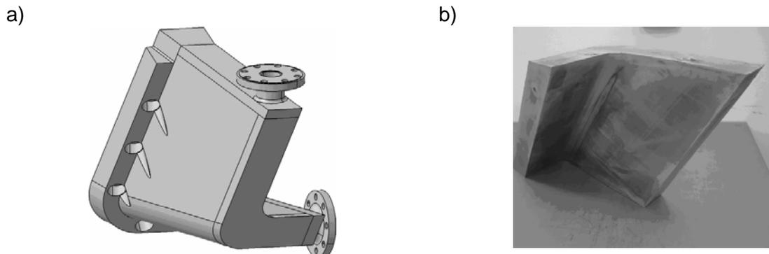
FIG. 6. a) BSM corner prototype model and b) the double wall body manufactured by HIP.
