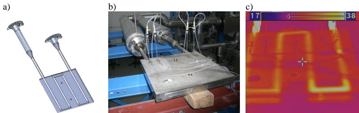
FIG. 3. Mock-up with drilled cooling lines: a) Catia-model, b) mock-up with connections to cooling circuit and c) thermal mapping.
