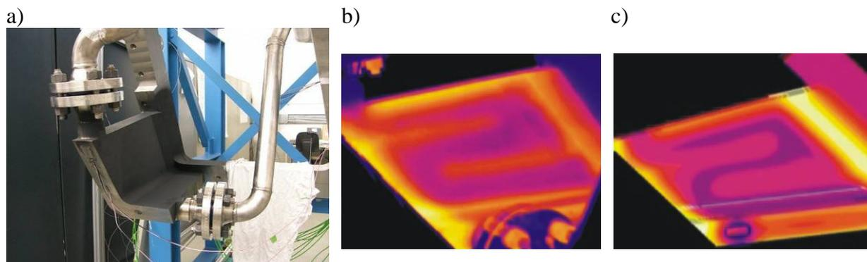
FIG. 7. a) BSM corner prototype mounted to the flange prototype and connected to water circuit, b) temperature map from infrared measurement and c) from simulation (after 80s shock cooling).
