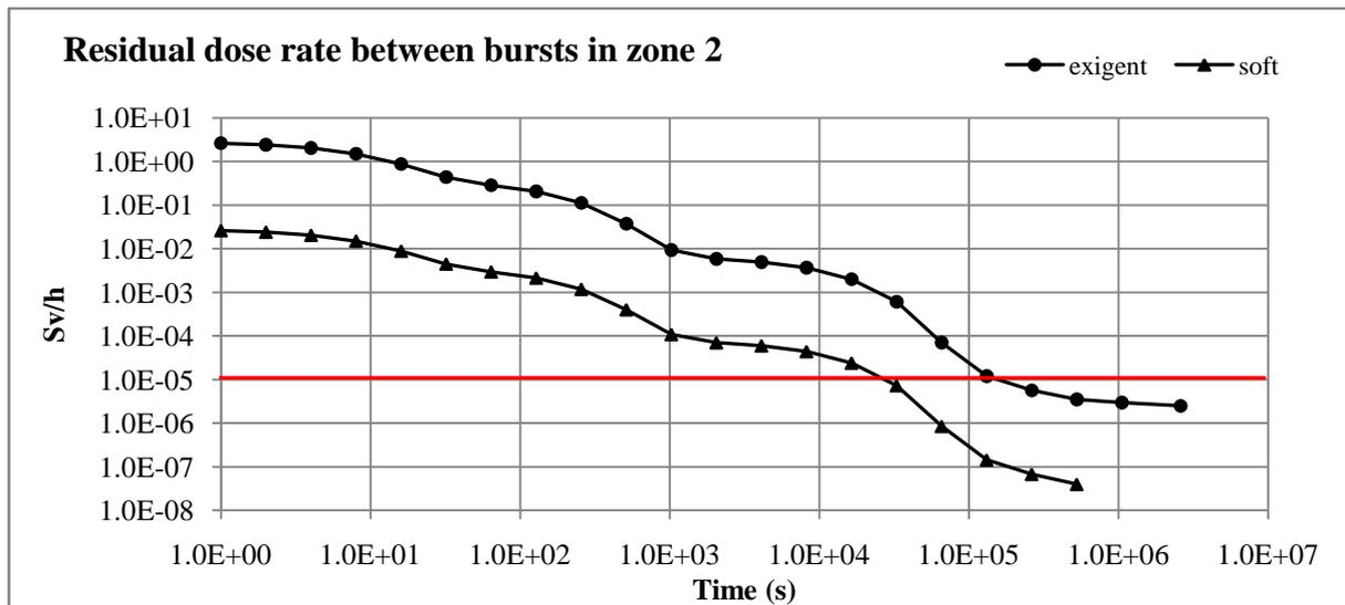
Figure 3: Time evolution of the RDR in zone 2 comparing two irradiation scenarios
